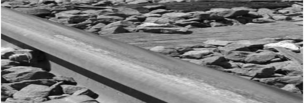
Figure 3.9. Longitudinal scuffing apparent in friction modifier in low rail of 200 m radius curve [30].
