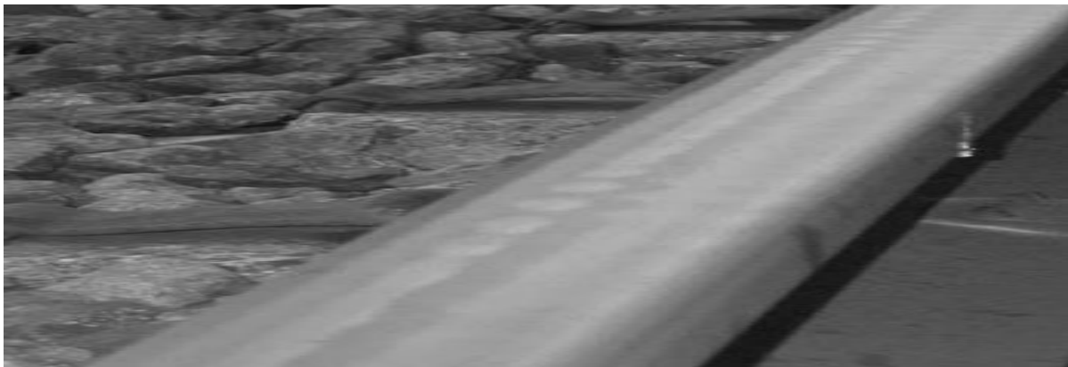
Figure 3.6. roaring rail from a metro system and from the UK main-line railway [27]
