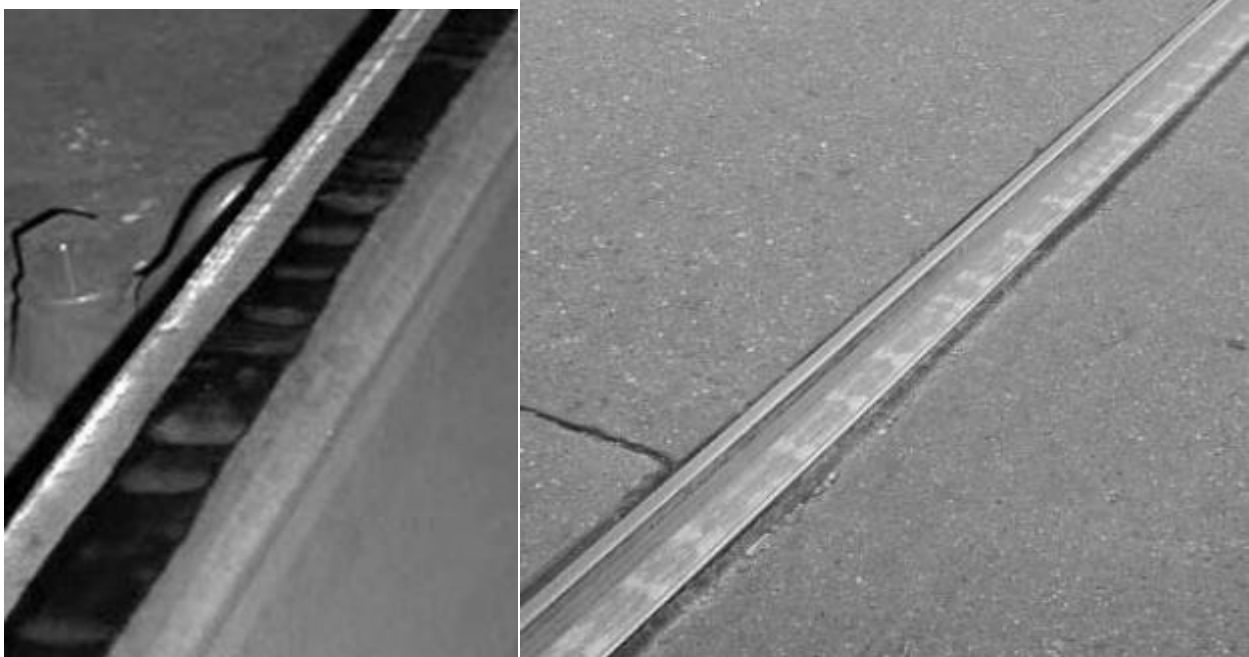
Figure 3.4. a) ‘Pinned–pinned resonance’ and ‘P2 resonance’ b) P2 resonance’ corrugation on a tram system corrugation on the same rail[26].
