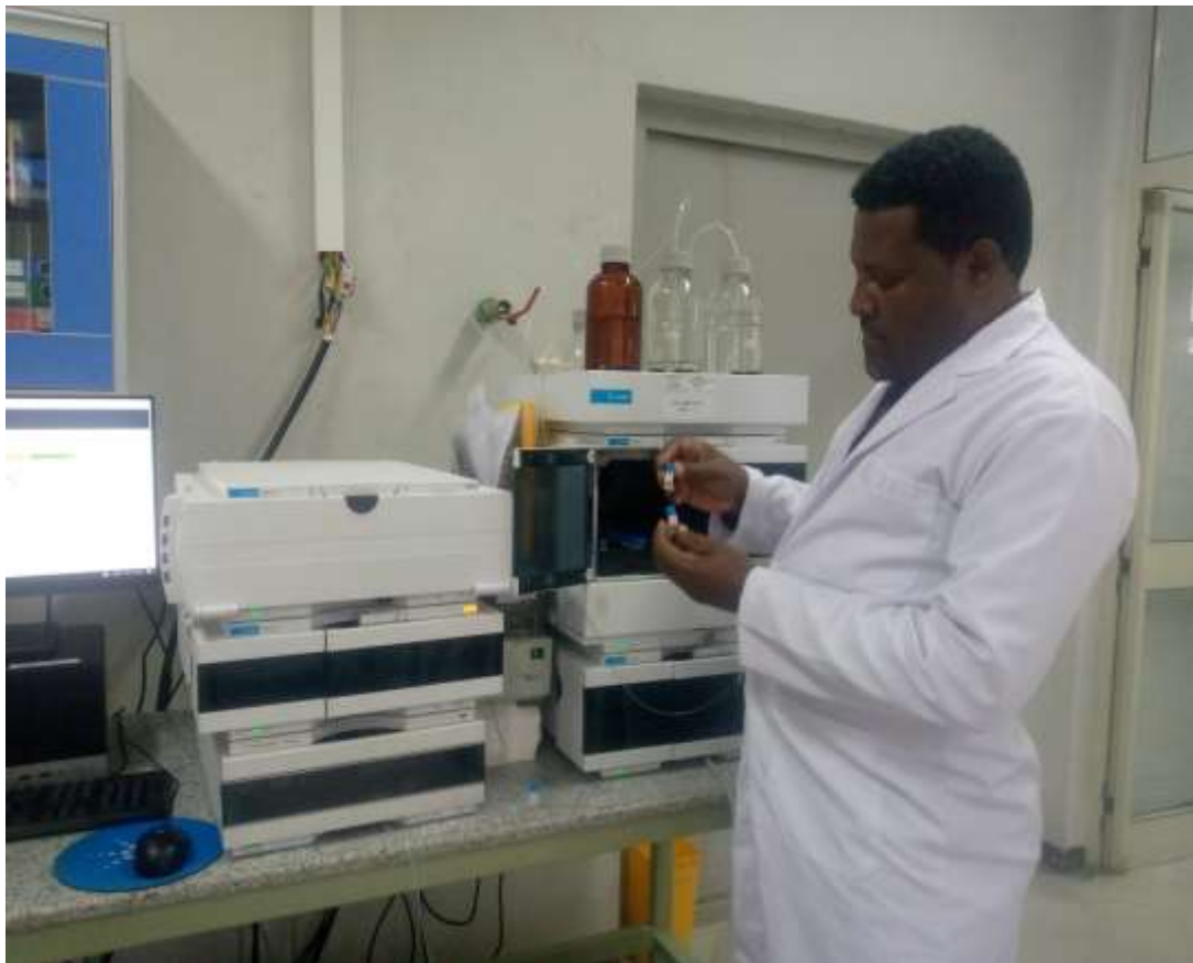
Figure 8. Photo taken during sample analysis (samples in sample vials ready for HPLC machine reading)
