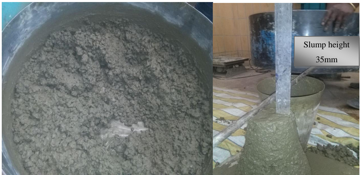
Figure 4.3: Prevailing Concrete Mix and Slump test of 20% Cement partial replacement by Fly ash and Basaltic dust
