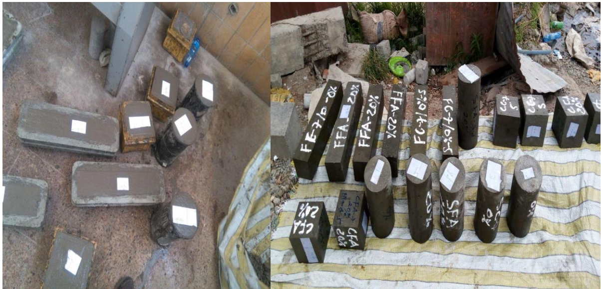
Figure 4.4: Concrete samples preparation and its curing scenario with different replacement amount of wastes (fly ash and basaltic dust)
