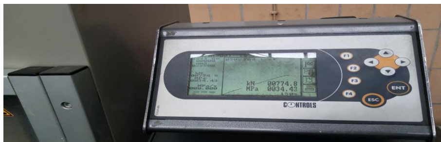
Figure 4.5: Compressive Strength of the Conventional Concrete at 7 days
