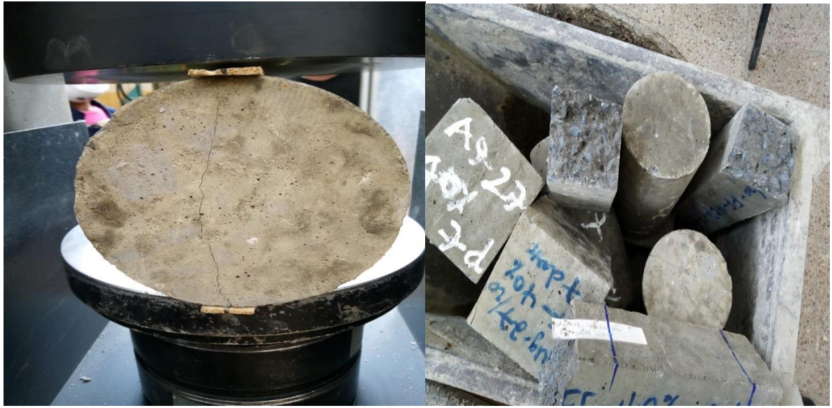
Figure 5.5: Prevailing Cubic, Flexural and Split Tensile Strength Samples after crushed/smashed
