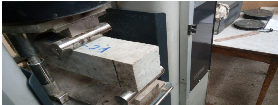
Figure 4.7: Flexural Strength of the Conventional Concrete at 7 days
