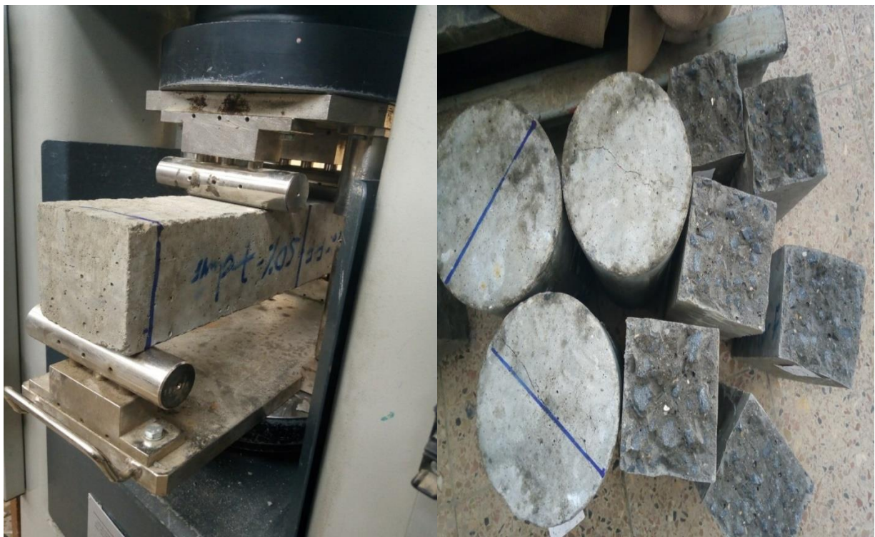
Figure 4.9: Prevailing Flexural and Split Tensile Strength Samples after crushed/smashed
