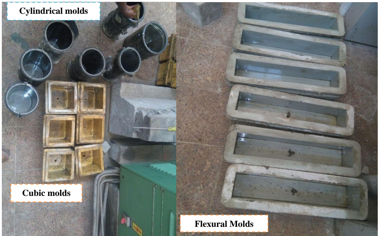
Figure3. 7: The molds used for the prevailing study, (108) samples were prepared
