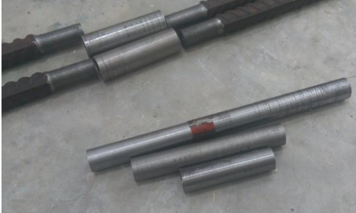
Figure 3.2: Coupler internal and external reinforcement thread (Manufacturing external and internal thread from Debre Birhan University Mechanical Lab)
