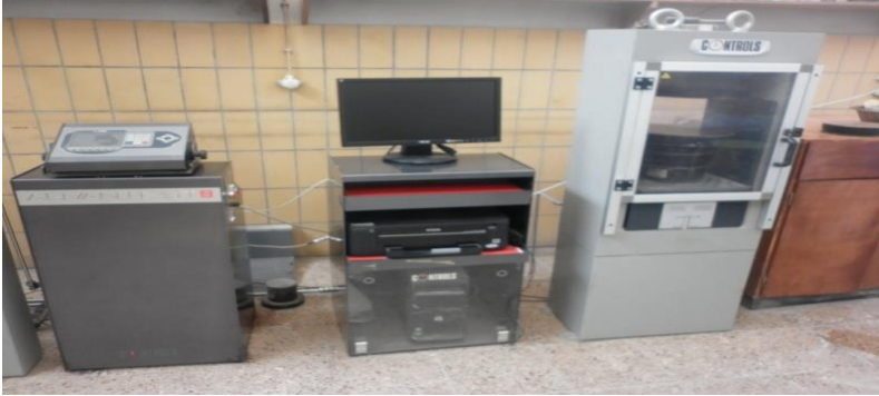
Figure 3.6: Concrete Compression Cubes Test Machine (From Adiss Ababa University Institute of Technology Civil Lab)
