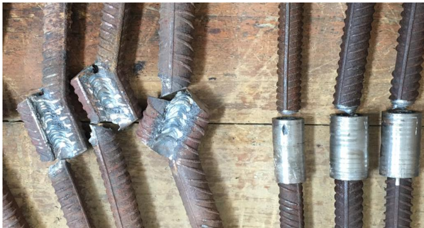
Figure 4.5: Welding and Coupler splice after tensile test
