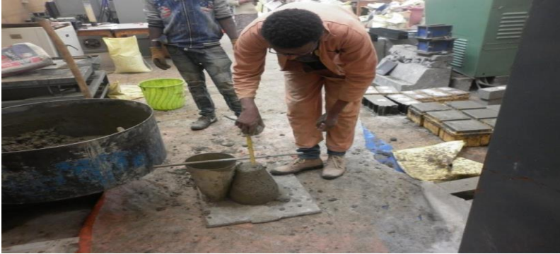
Figure 3.4: Slump test (From Adiss Ababa University Institute of Technology Civil Lab)
