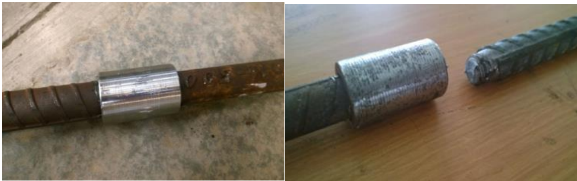
Figure 2.6: Coupler Splice before and after Test [39]
