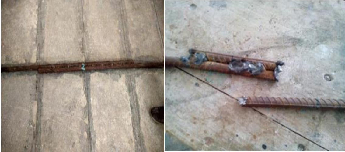
Figure 2.5: Welded Splice before and after Test [39]
