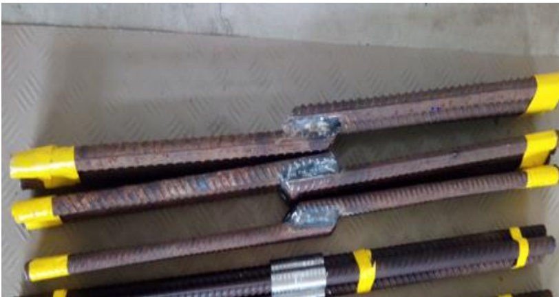
Figure 4.2: Lap Welding Splice Reinforcement steel (Photo Lab Tensile Test Reinforcement)
