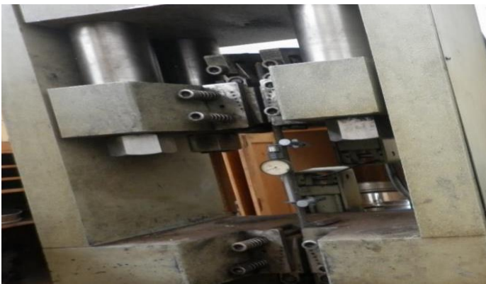
Figure 3.3: Reinforcement Bar Tensile Test Machine (From Adiss Ababa University Institute of Technology Civil Lab)
