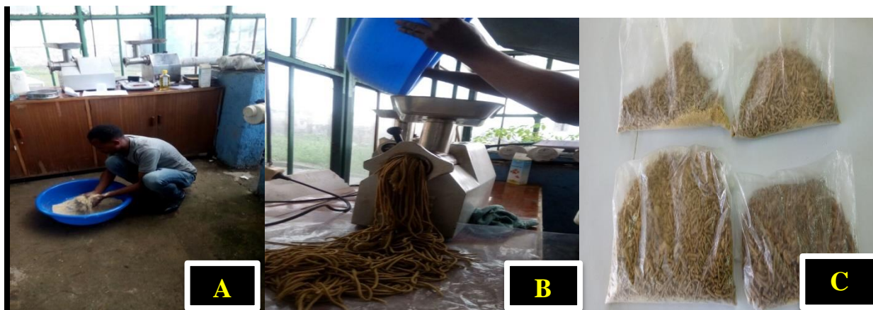
Plates 6: Mixing of feed ingredients (A) pelleting of experimental diets through an electrical meat mincer (B) and packing in a polyethylene bag (C)
