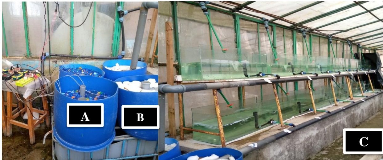
Plates 1: Filtration components of recirculating aquaculture system, (biological filtration-A), (mechanical filtration-B) and twelve experimental aquaria (C)
