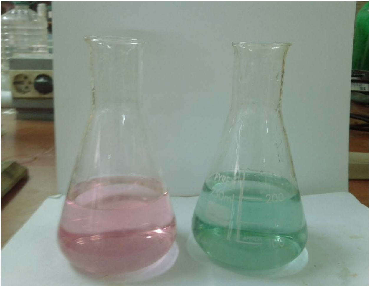
Fig. 4. Leaf N analysis, showing a pink color to the left after titrated with 0.1N H 2 SO 4 .
