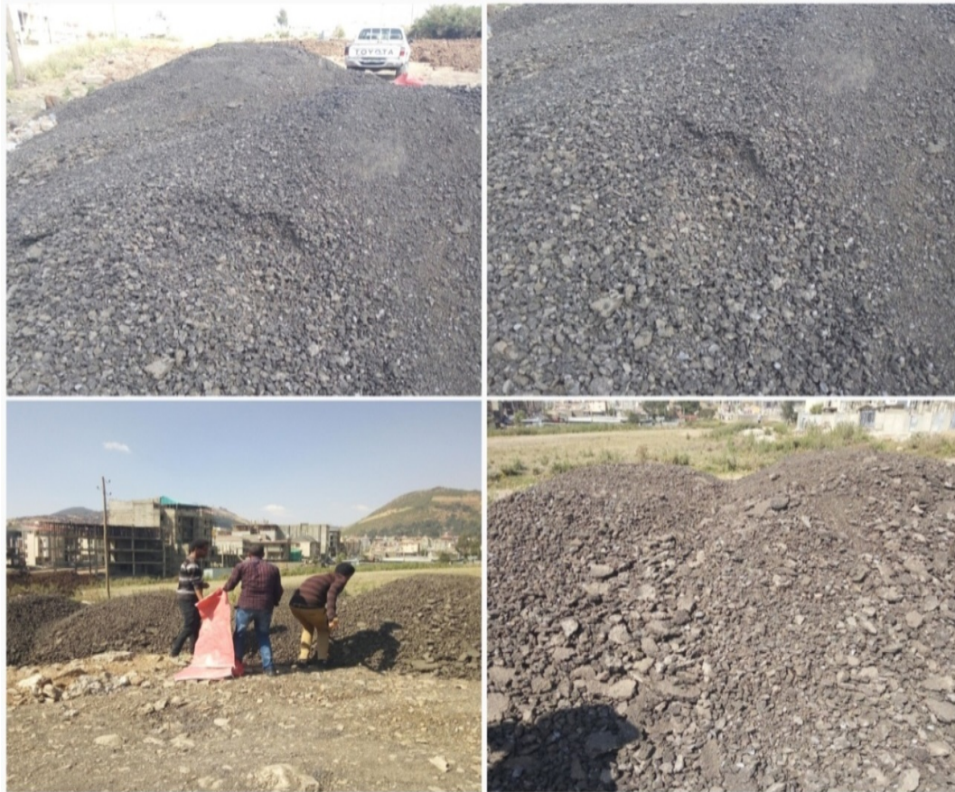
Figure 3.1: Sampling of RAP material at Ayertena Alembank
