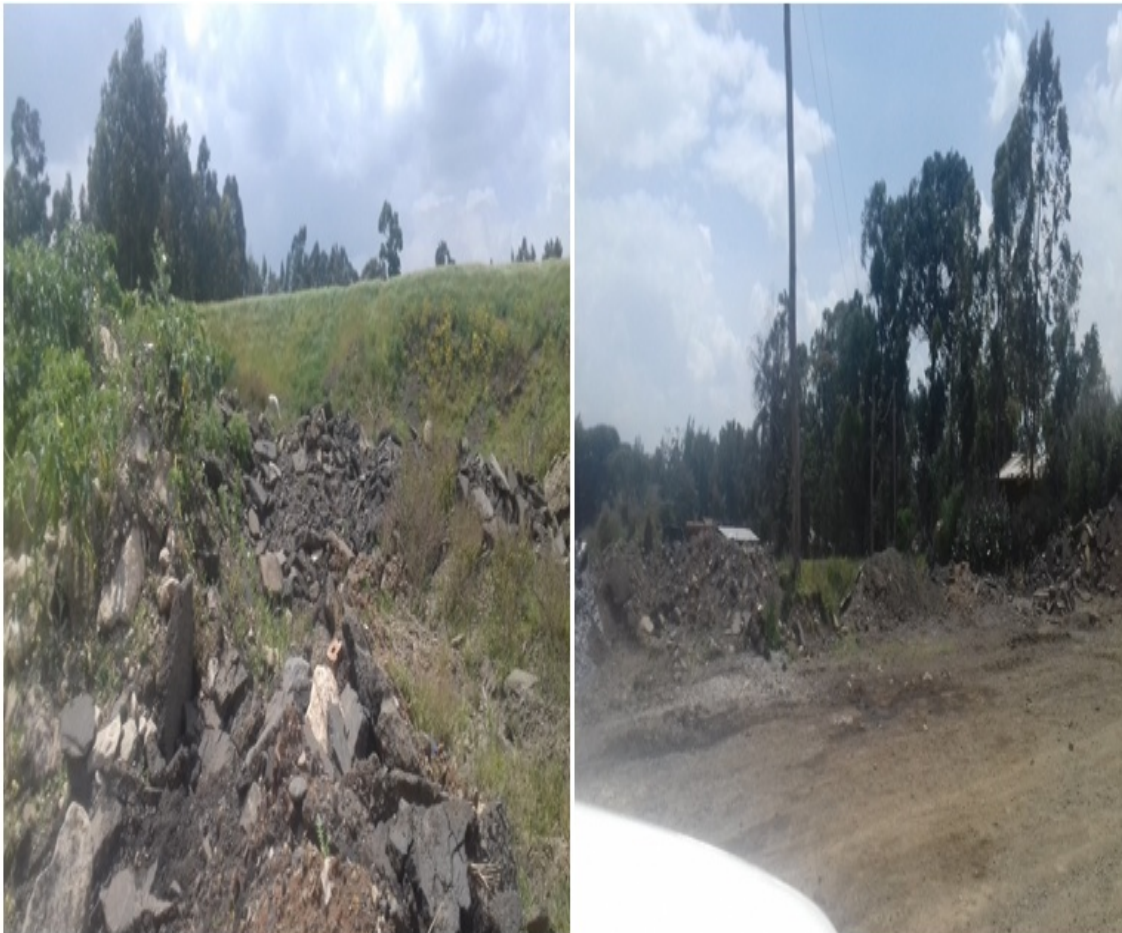
Figure 2.2: Multiple source RAP pile with dirt contamination (photo at Kality Korki quarry site)
