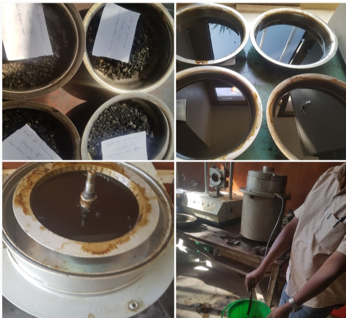
Figure 3.3: Extraction of RAP aggregate using centrifugal method (photo at AACRA central laboratory).
