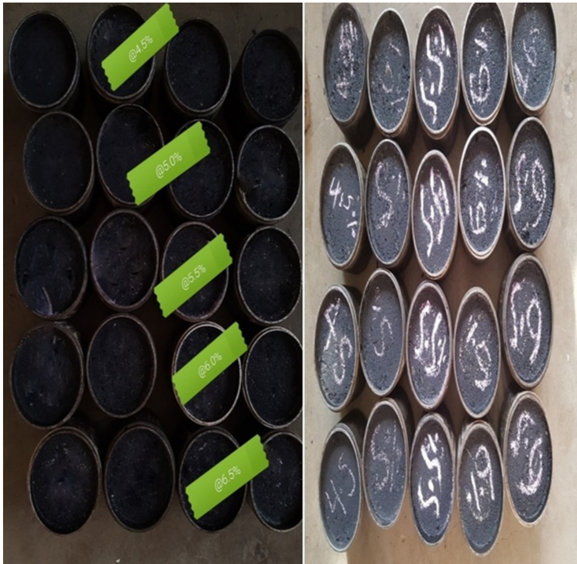
Figure 3.7: Compacted Marshall specimen at different bitumen and RAP content (photo at AACRA Central Laboratory)
