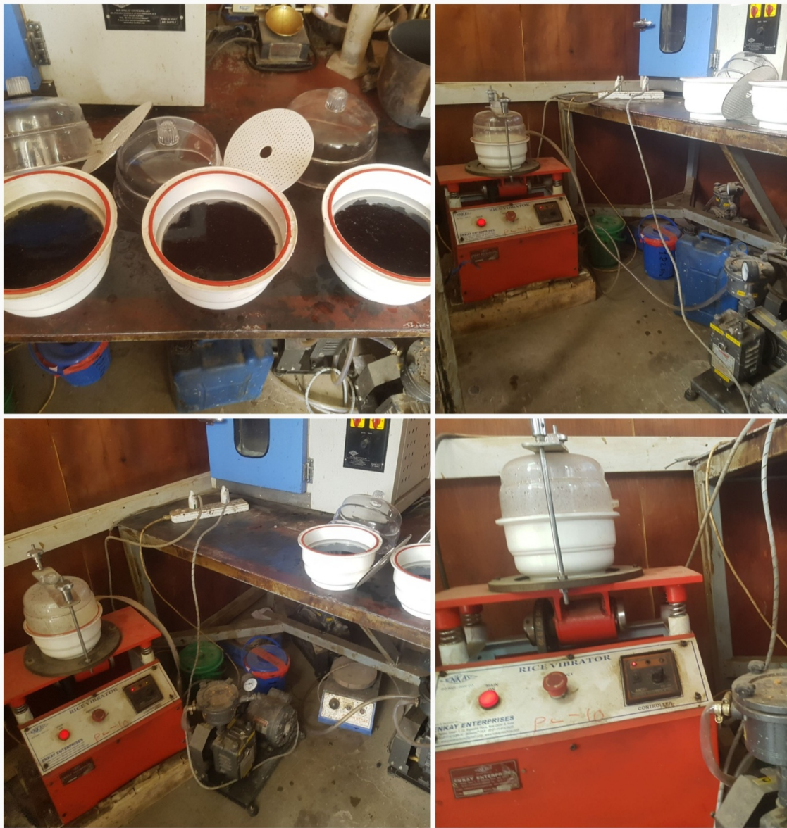
Figure 3.2: Determination of maximum theoretical specific gravity ( G_{mm} ) of RAP (Photo at AACRA Central Laboratory)
