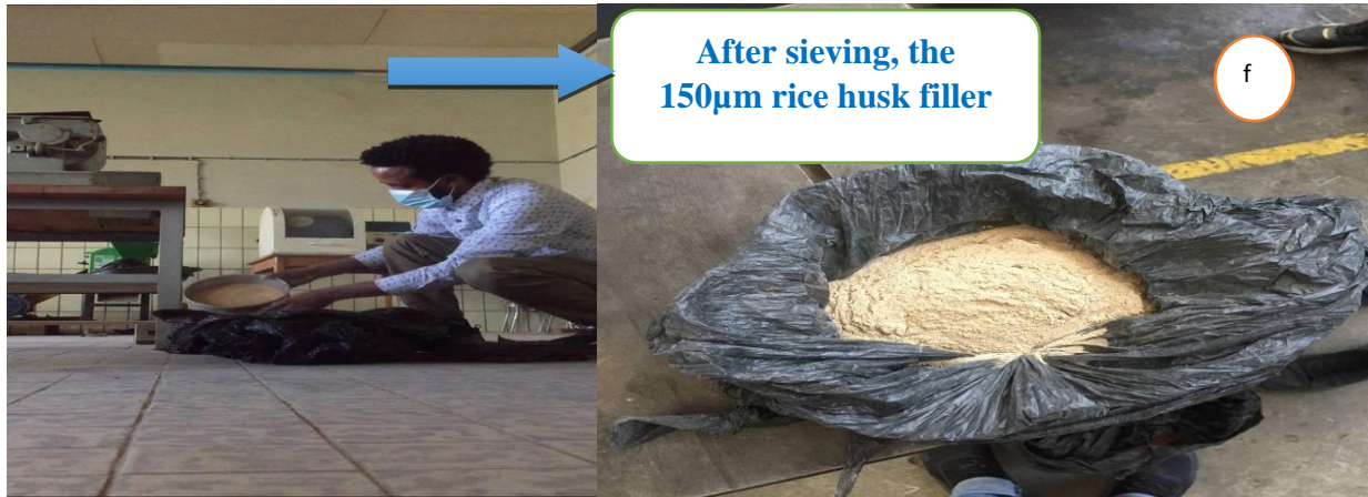
Figure 3.2: a) Unmilled Rice husk, b) glass fiber and c) sisal fiber d)milling Rice husk e).150mm sieve f)seived 150µm filler respectively:
