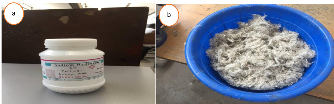
Figure 3.3: a) sodium hydroxide b) treated and washed sisal fiber
