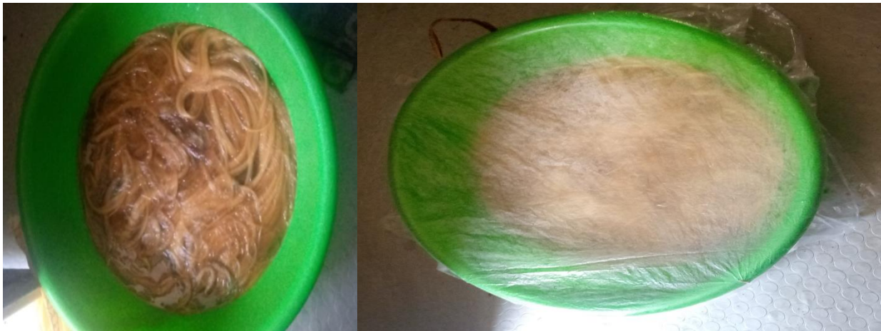
Figure 18 Soaked sisal fiber in NaOH solution and cover by plastic cover
