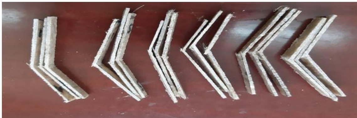
Figure 39 Specimens after flexural deformation
