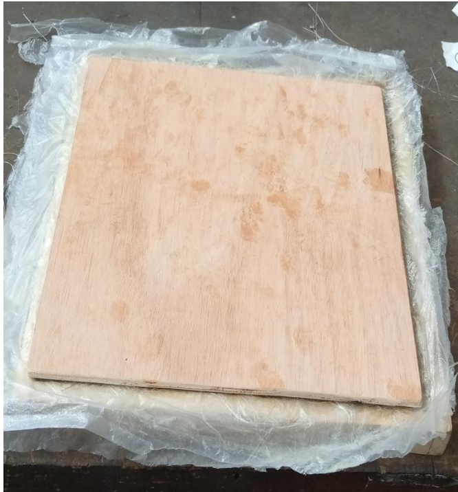
e) Placing fiber and matrix in the mold
