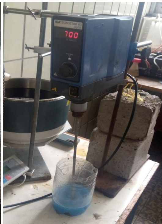
d) Mixing \text{Al}_2\text{O}_3 and polyester resin
