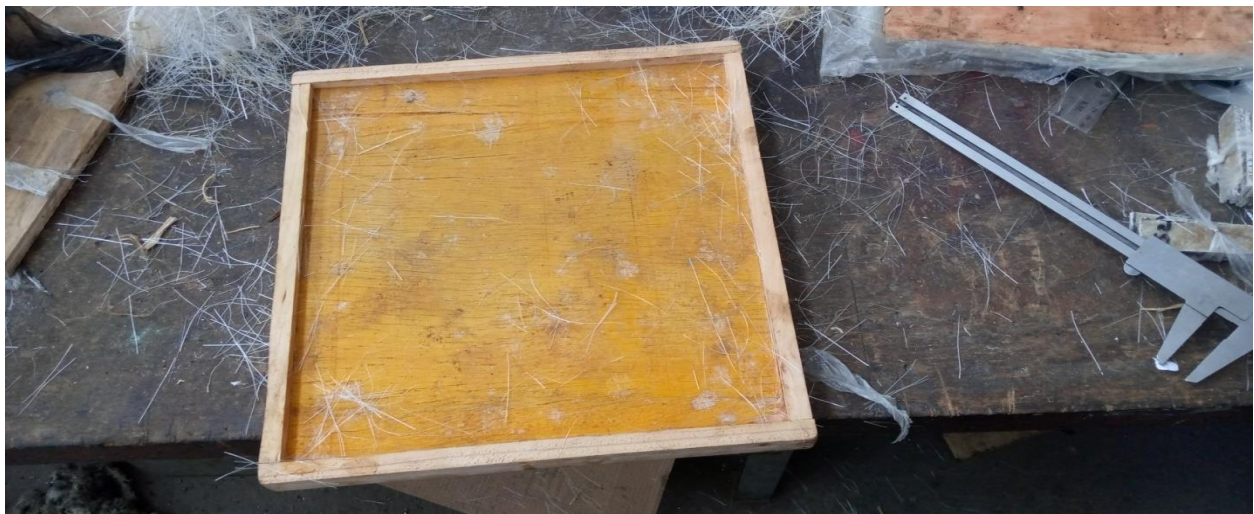
Figure 14 Prepared wooden mold to fabricate the composite
