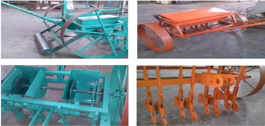
Figure 13 Teff Row seeder machine introduced by Ethiopian Institute of Agricultural Research (EIAR)
