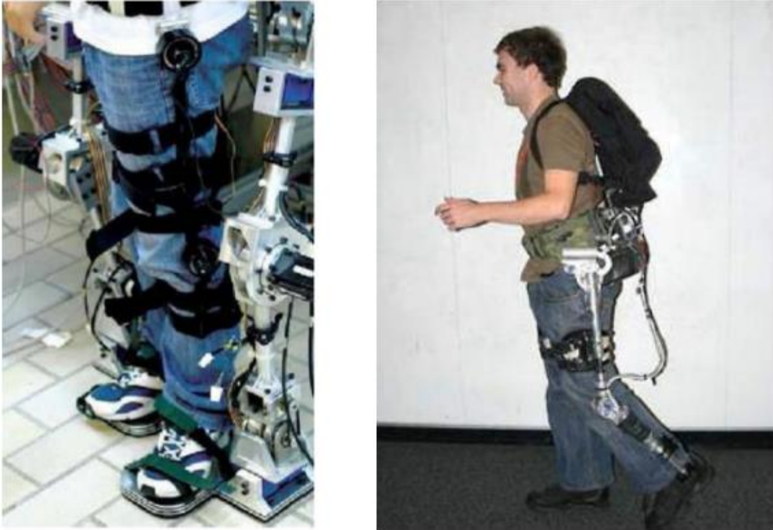
Figure 2.4: The Lower Extremity Exoskeleton (LEE) (left) and Under-actuated exoskeleton with passive elements (right)
