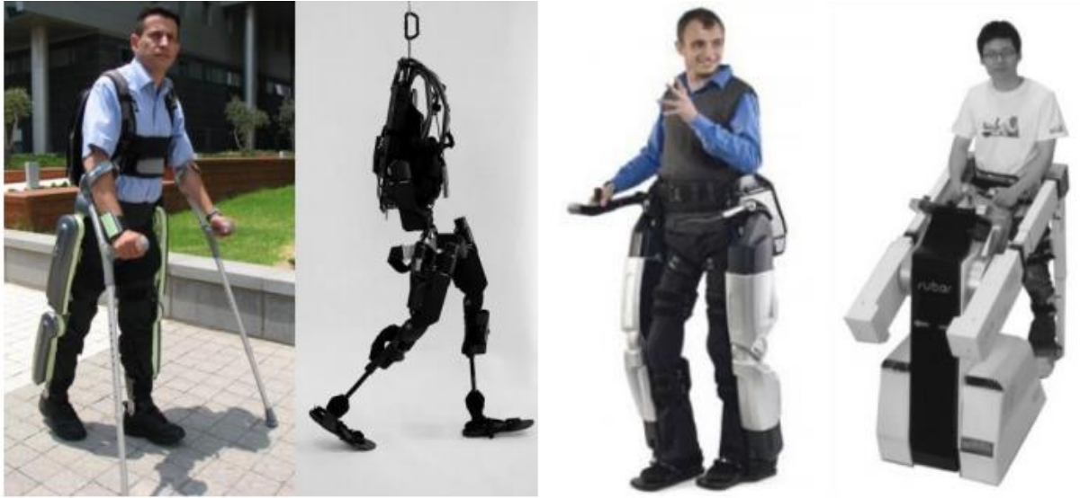
Figure 2.2: From Left to right, ReWalk by Argo Medical technologies; Esko by Berkeley Bionics; REX by Rexbionics ; and SUBAR by the University of Sogang
