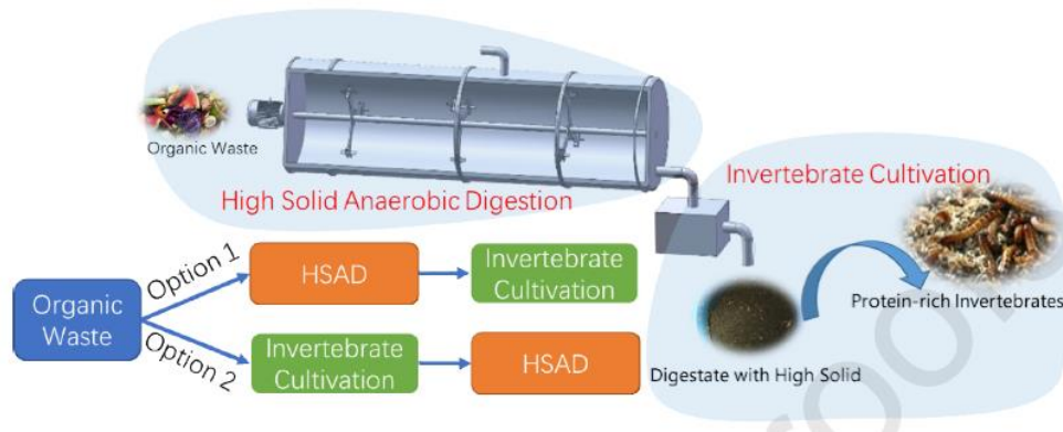
Figure 30: Two options for the integration of high solid anaerobic digestion (HSAD) with invertebrate cultivation
