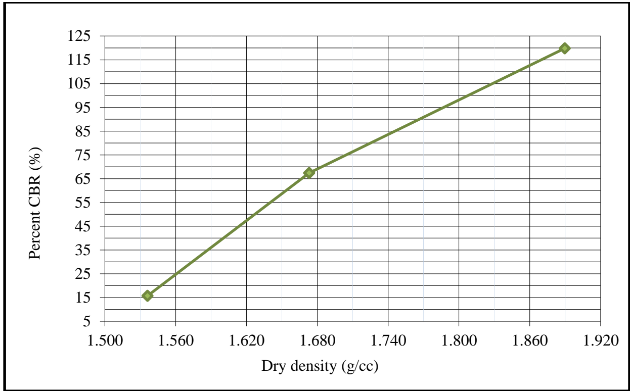
Figure C – 6: Dry Density Vs percent CBR of cinder with 20 % fine-grained soil
