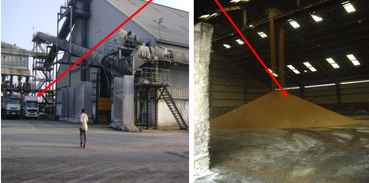
Figure 4.3. Loading and storing of fertilizer to the trucks and silo at the same time
