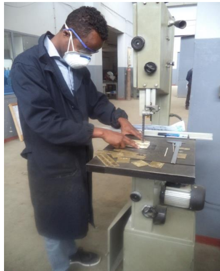
Figure 24. Sample preparation using band saw
