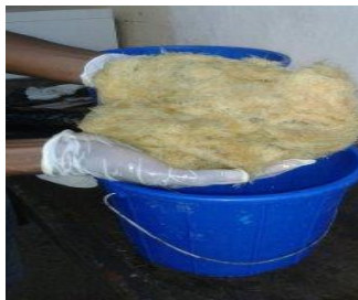
Figure 17. Pure sisal fiber after mercerization
