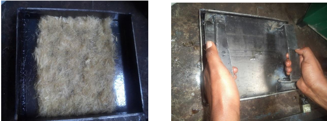
Figure 21. Sisal fiber- epoxy resin mixture in the mold surface at AAIT lab
