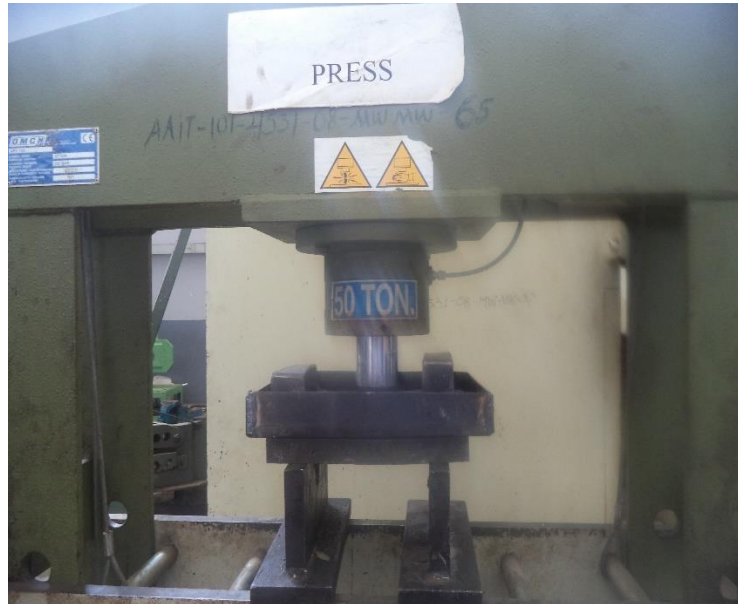
Figure 22. Standard Hydraulic Press for curing
