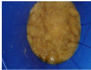
Figure 16sisal fiber soaked in NaOH solution for 24hrs
