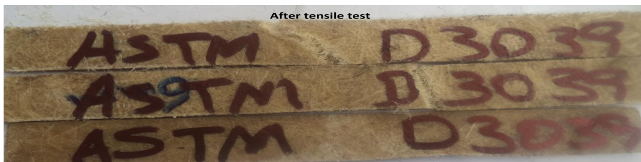
Figure 30. Sisal fiber reinforced epoxy composite material after Tensile Test
