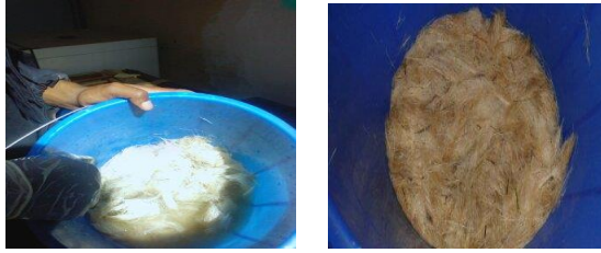
Figure 14. Chopped sisal fiber with in distilled water at 80 0 c for 1 hrs
