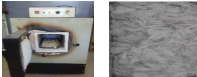
Figure 15. Sisal fiber dried with inside the oven and after the oven
