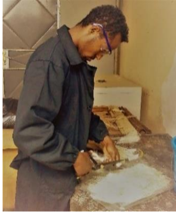
Figure 13(a) chopping the fiber (b) the chopped sisal fiber
