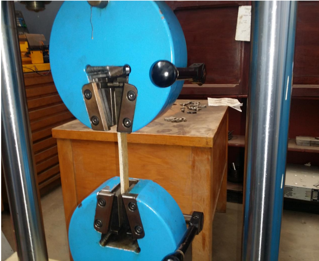
Figure 29. Typical specimen under tensile strength test
