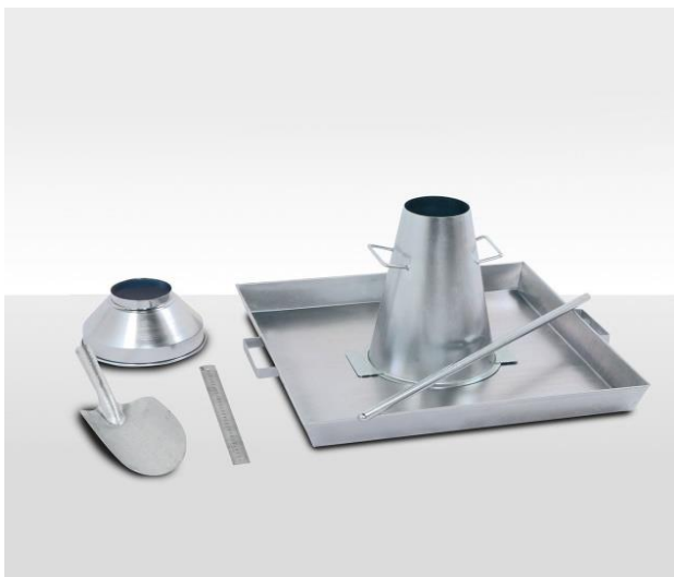
Photo: Slump Cone apparatus
