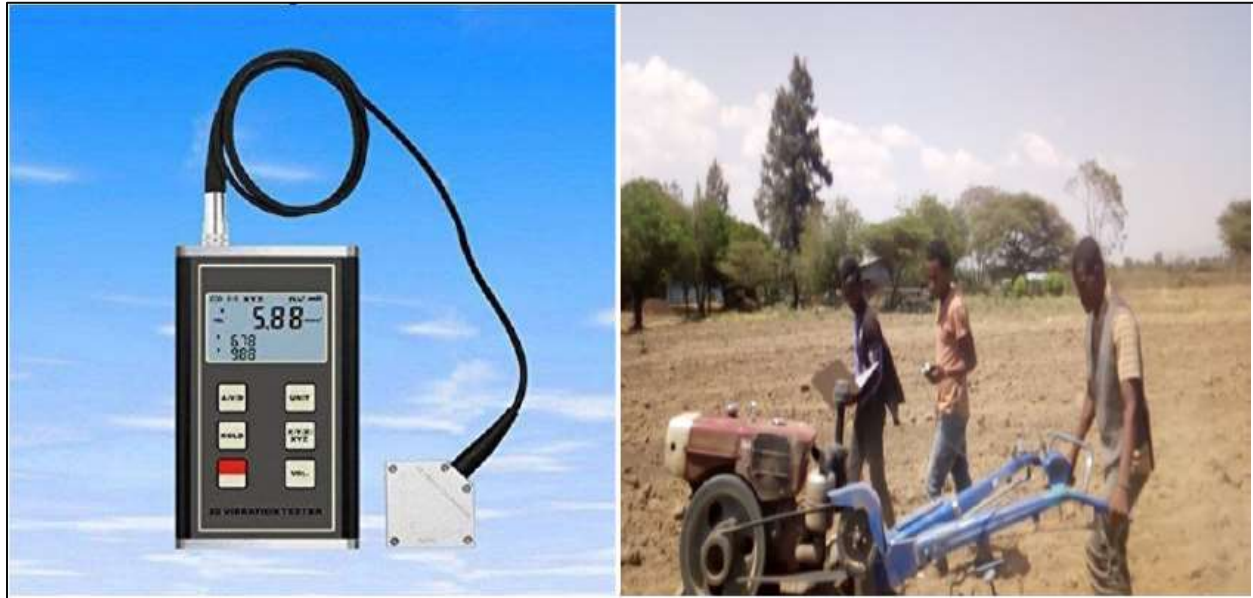
Figure 2- 10 A VM-6380 3-Axis 3D Digital Vibration Meter Tester and measurement of vibration
