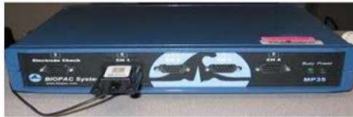
Four Channel Data acquisition Unit MP 35 (Biopac Systems Inc, USA)
