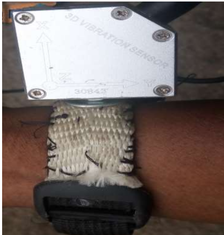
Figure 4- 4vibration measurements at the hand of single axle tractor operators
