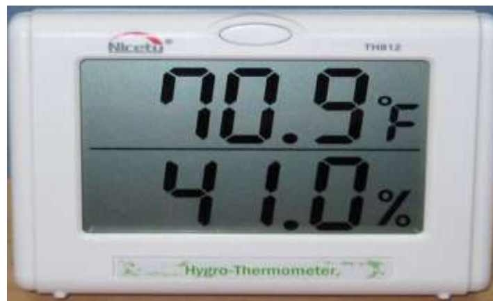
Figure 2- 6 Large Digital Temperature Humidity Meter - Hygrometer and Thermometer (© 2010 CarstanFranke)
