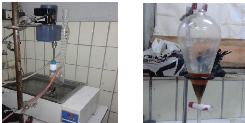
Figure 3.6 Transesterification reaction & Separation of biodiesel from glycerol
