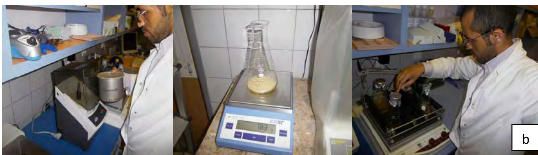
b. Collecting and weighing specimen's powder and extracting it using laboratory shaker
