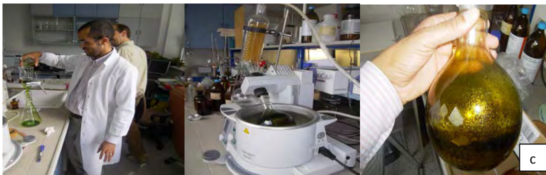
c. Filtering, evaporating and collecting final extracts
