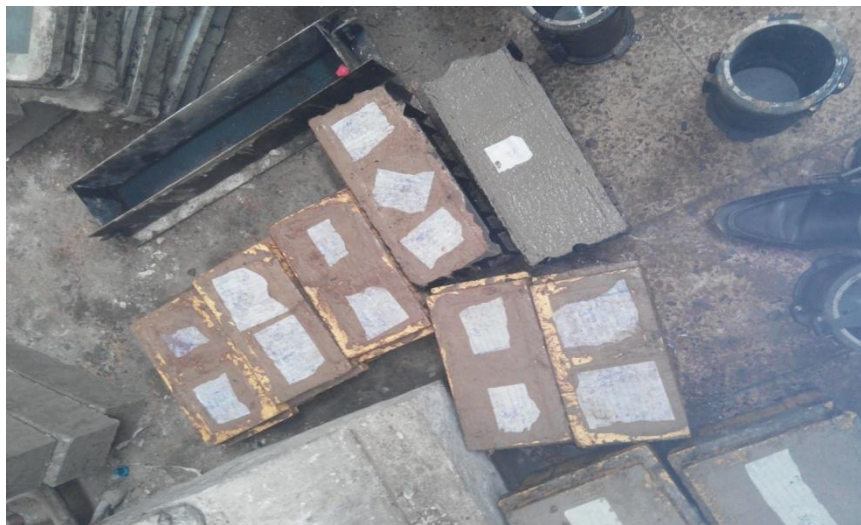
Figure 3.2: Concrete casted from 10cm x 10cm x 10cm cubes
