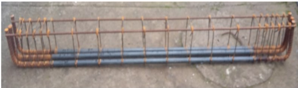
Figure 3-12: Reinforcement cage of full span unbonded beam
