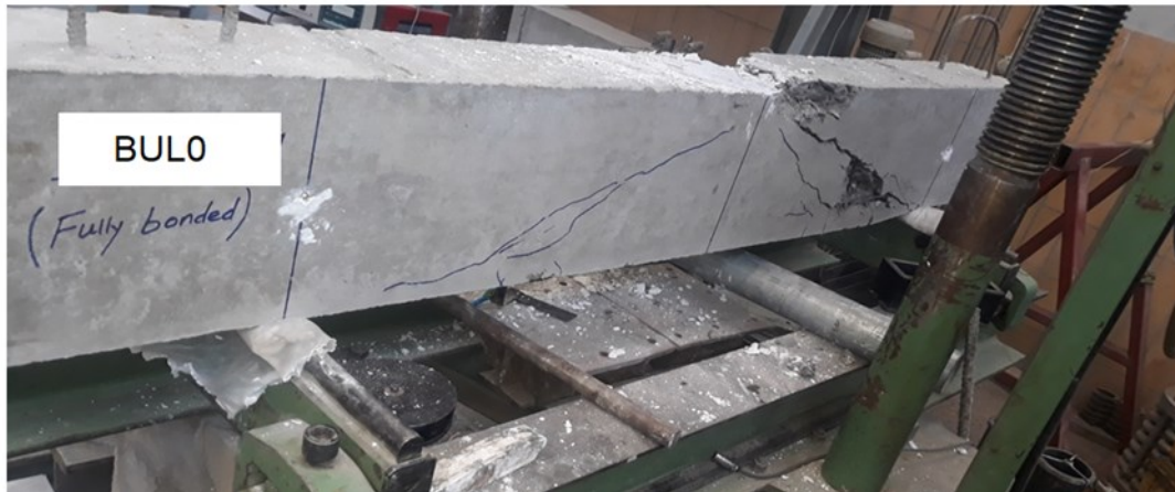
Figure 5-1: Failure mode of BULO
