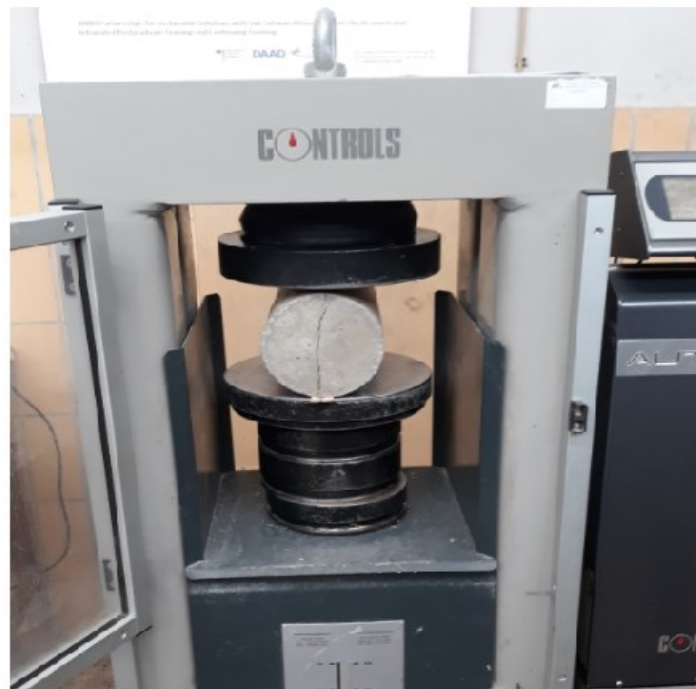
Figure 3-6: Compressive strength test
