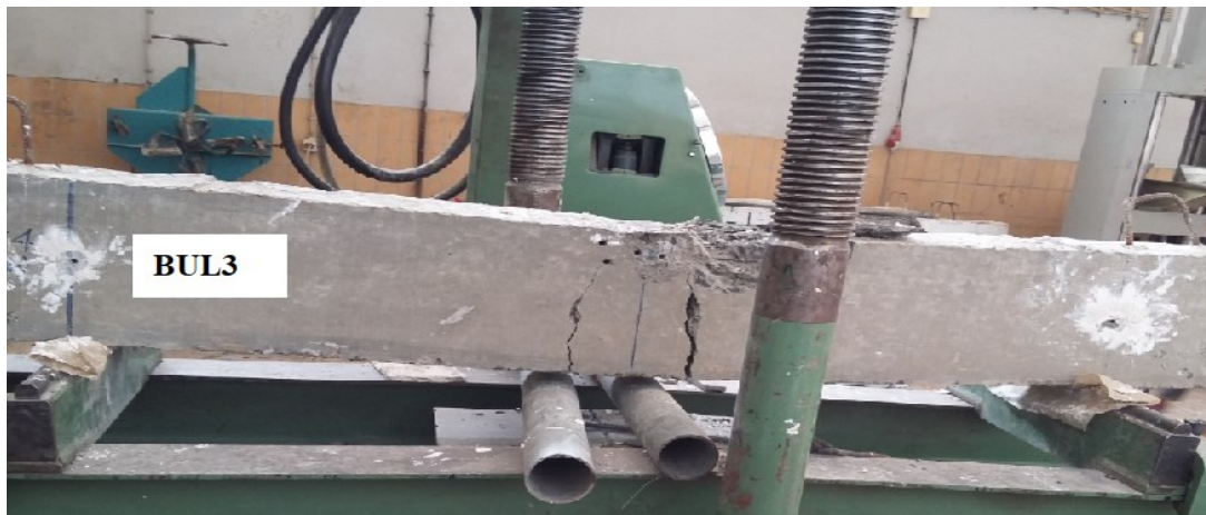
Figure 5-7: Failure mode of BUL3
