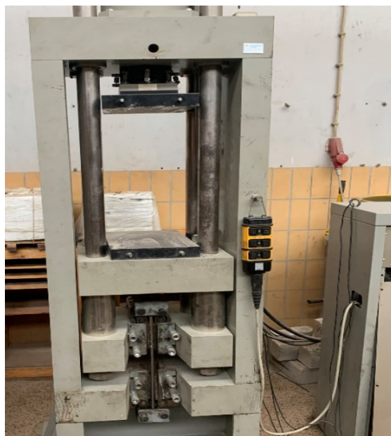
Figure 3-8: Tensile strength test of reinforcement
