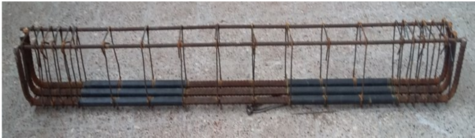
Figure 3-10: Reinforcement cage of one-third of the span unbonded beam
