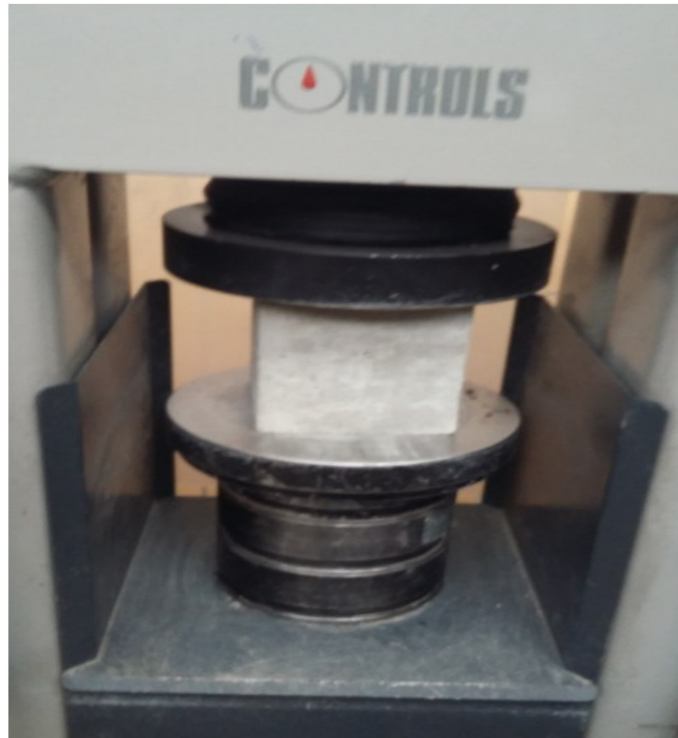
Figure 3-6: Compressive strength test
