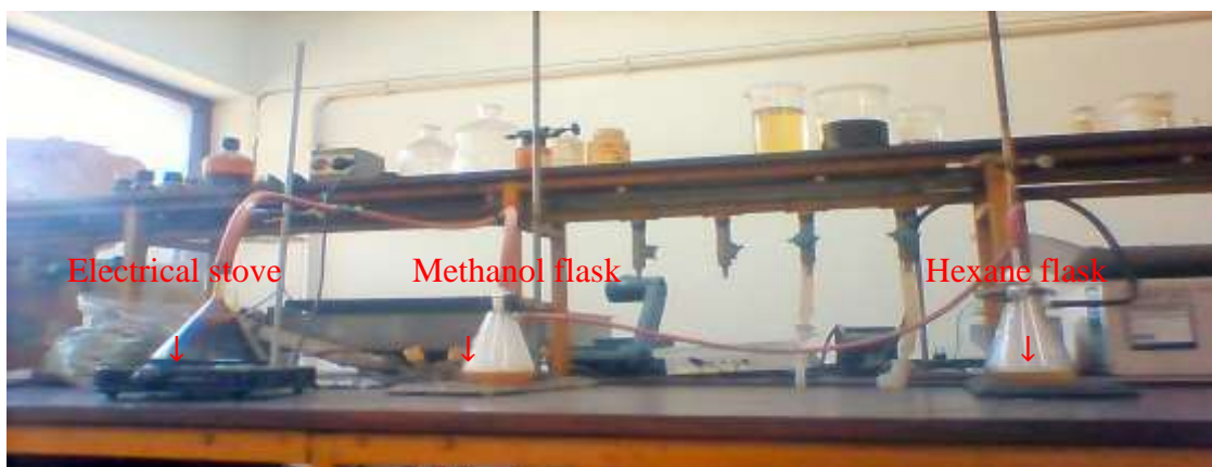
Figure 9: Smoke trapping and extraction system.
