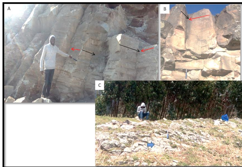
Fig.3.20. Close view of systematic joints with two sets of joint in rhyolite lava flow (A), arrows show opposite joint faces to indicate two joint sets; trachyandesite(B); and Polygonal joint in trachybasalt (C).
