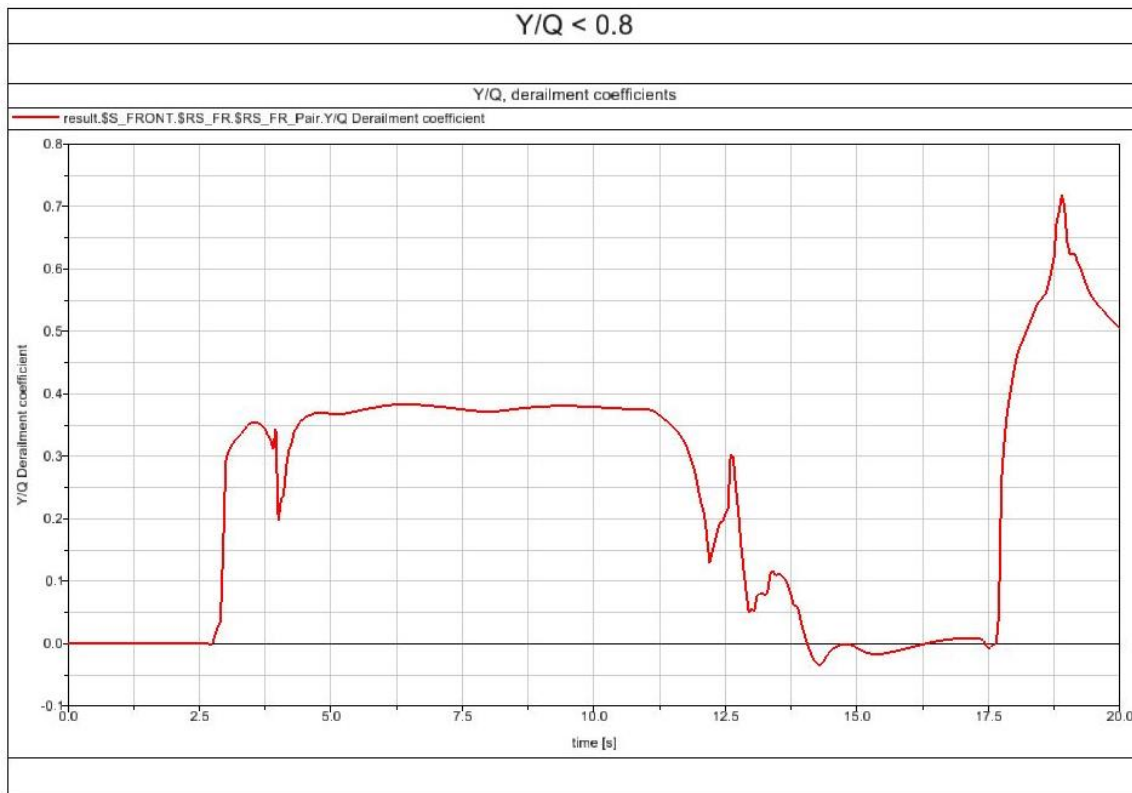
Figure 5. 2 The graph of derailment coefficient before wheel-rail defects
