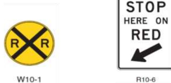
Figure 2-5 Advance warning signs (W10-1) and Stop Here on Red
