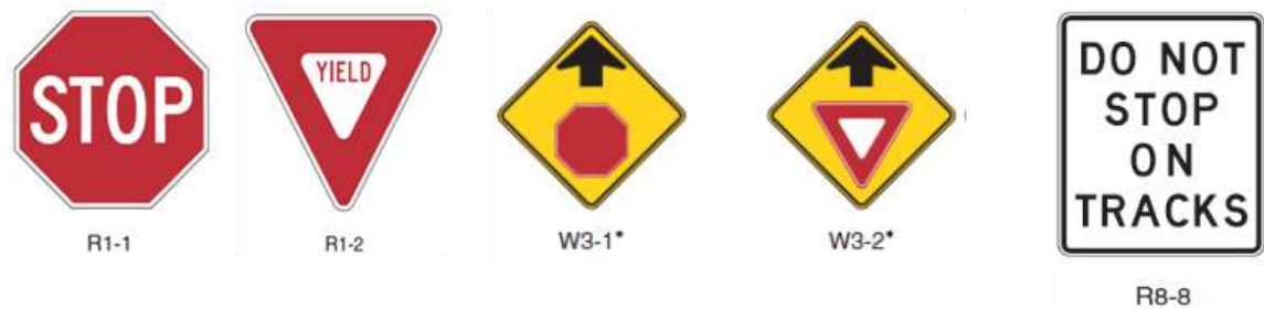
Figure 2-4 Stop (R1-1), Yield (R1-2), Stop Ahead (W3-1), and Yield Ahead (W3-2) signs
