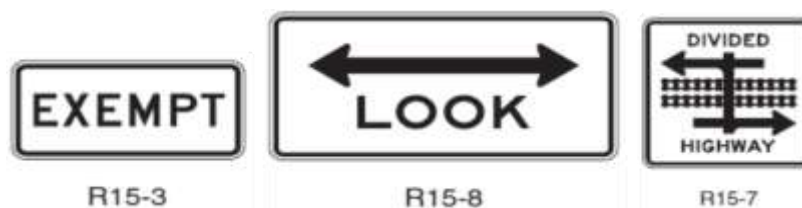
Figure 2-6 Supplemental passive traffic control signs
