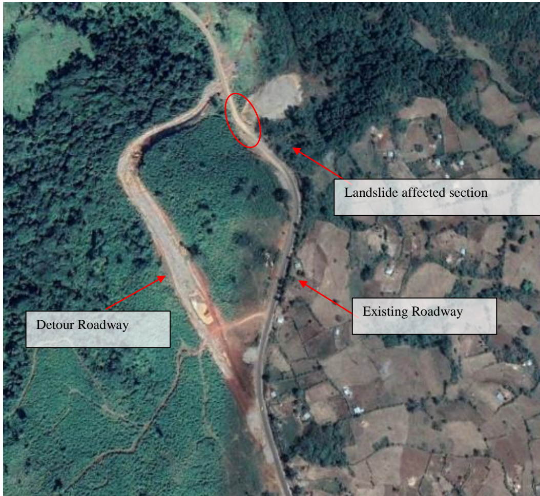
Figure 4-7: Existing and new detour roadways at 36+720 (Gechi) [Source – Satellite Image by Google Earth]
