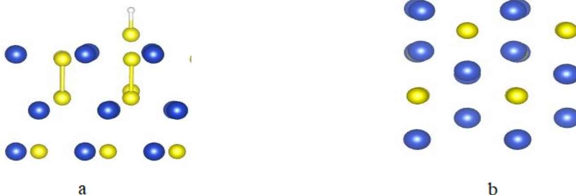
Figure 9 Geometry optimization plot of H adsorbed on the CuS (001) surface (a) View along y- axis (b) View along z- axis
