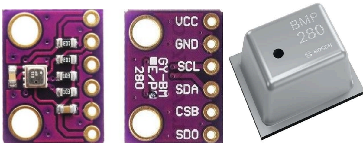
Figure 3-9: GY-BMP/E280 combined humidity, pressure, temperature, proximate altitude sensor module front (left), back side (middle) and IC package (right) [61].
