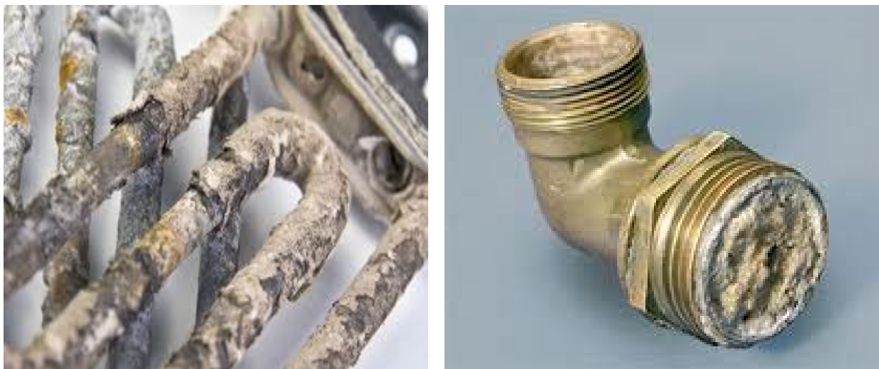
Figure 5-51: Effect of chalky ( \text{CaCO}_3 ) deposit on the heating element and tubes [102].
