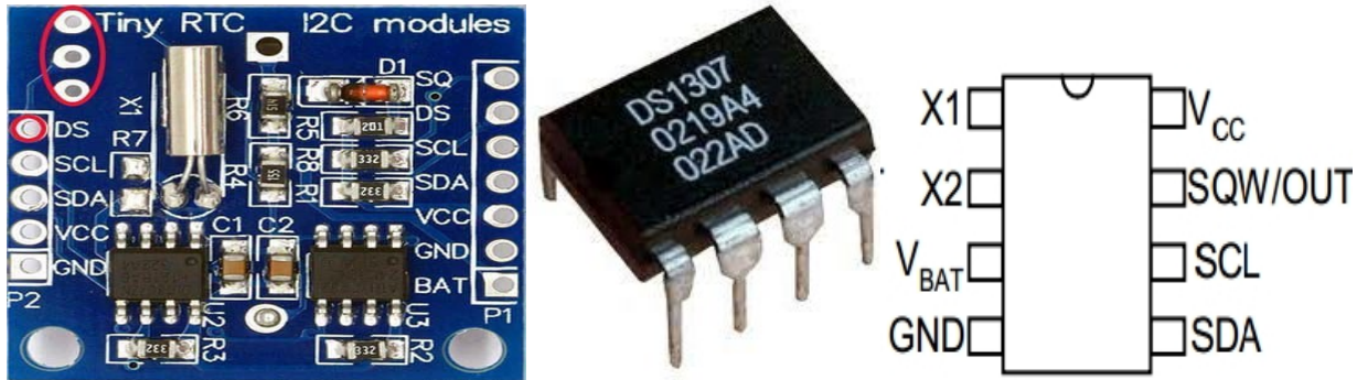
Figure 3-10: The DS1307 RTC module (left), DS1307 IC (middle) and DS1307IC pin description(right) [63].
