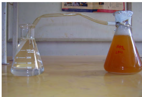
Figure 7. Experimental setup for batch fermentation
