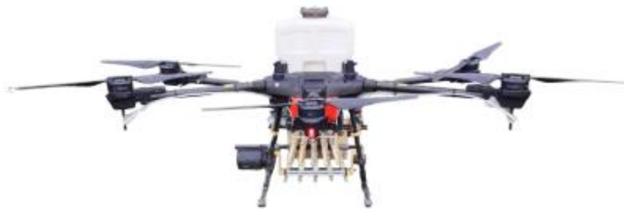
Figure 14. Potshot seeding drone (W. Liu et al., 2022).
