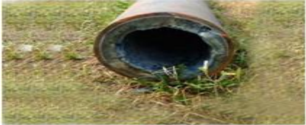
Figure 1 Struvite precipitation on pipe
