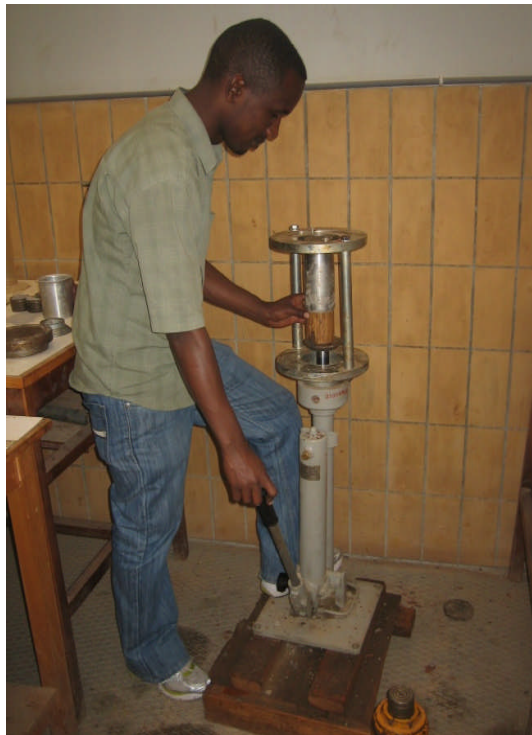
Figure B-2 Extruding undisturbed soil specimen from the sampling tube
