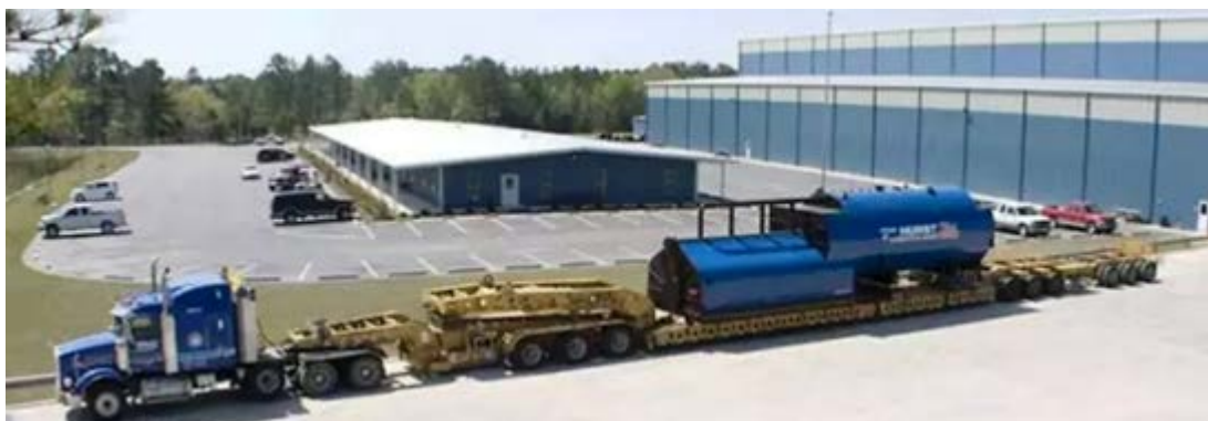
Figure 5.8: Transportation of Wood Biomass Boiler from Company to Port
