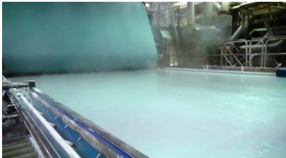
Figure 3.5: Sheet Formation and Dewatering Processes
