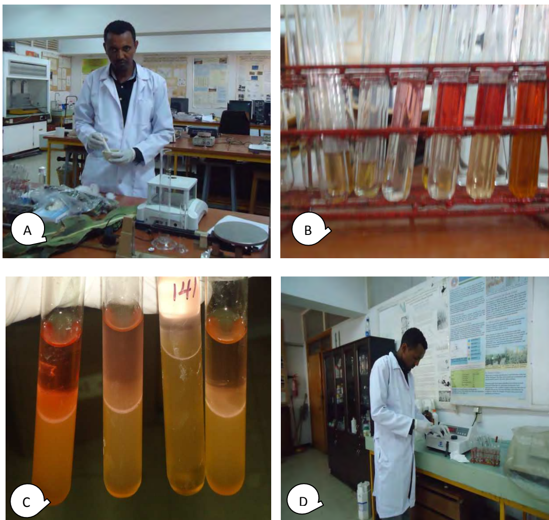
Fig.3. Determination of proline content, (A) Sample extraction, (B) Standard solution (C) Formation of two layers after toluene was added and (D) Reading the absorbance by spectrophotometer
