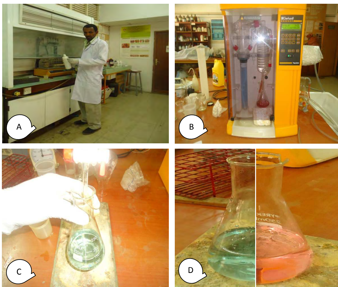
Fig.4. Determination of leaf nitrogen, (A) Digestion of a sample, (B) Distillation, (C) Titration and (D) colour difference after and before titration
