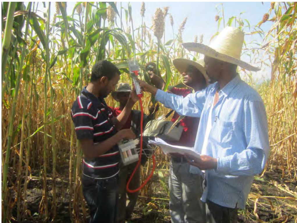
Fig.2. Measurements of leaf gas exchange using Lc pro+ photometer on the field at 30 DAF
