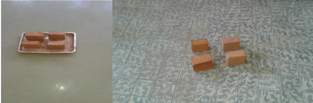
Figure 3.3 Air drying in the lab room before and after firing in the furnace
