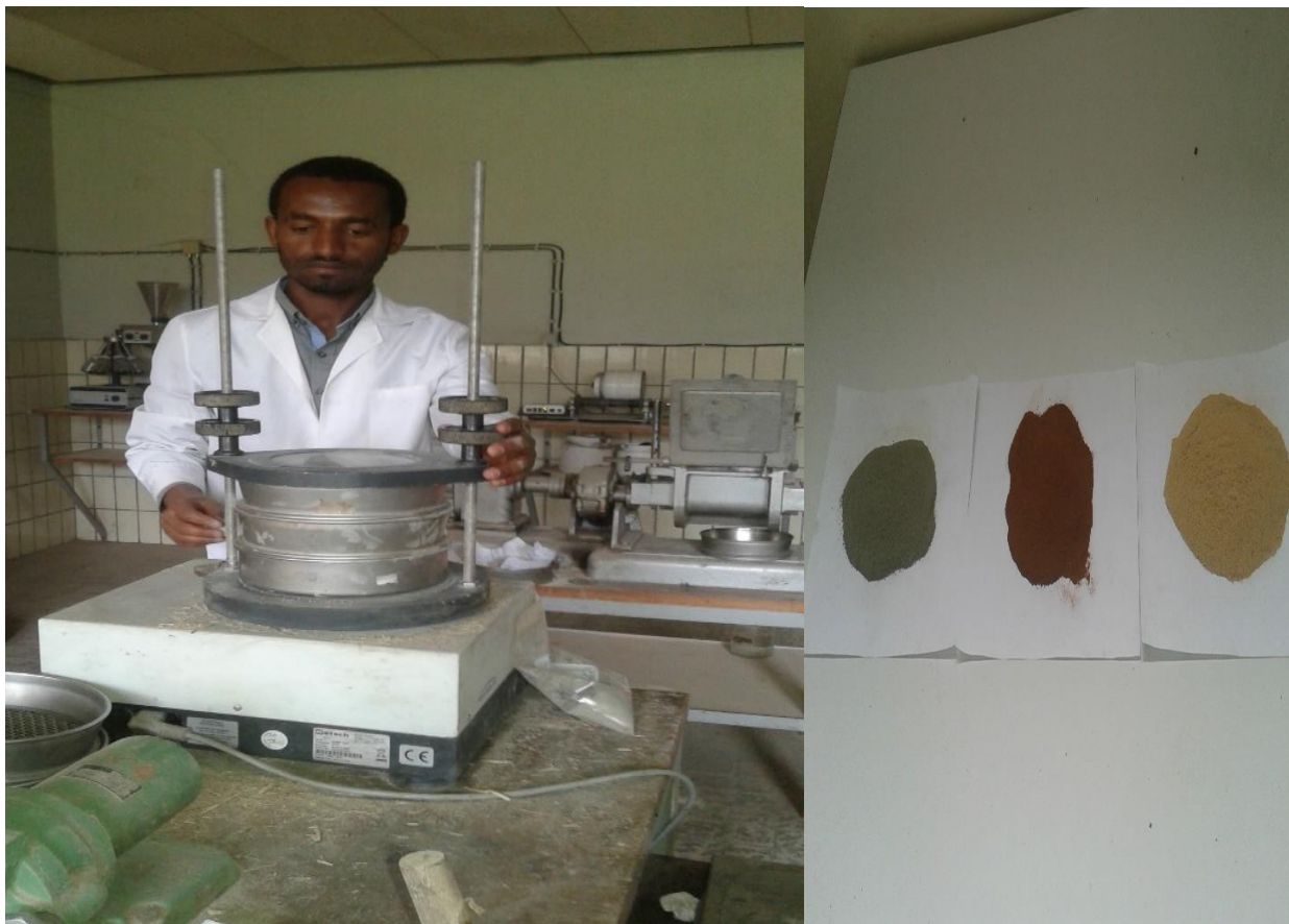
Figure A4. Oven dried textile sludge sample was crushed and sieved respectively
