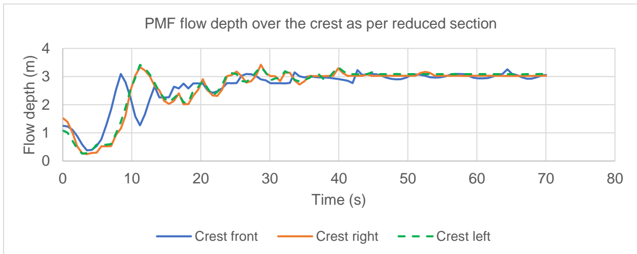
Figure 6- 7 PMF flow depth over the crest as per reduced section
