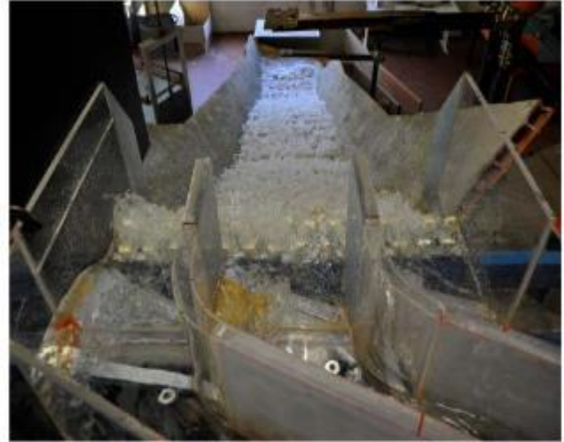
2 : Physical model along stepped chute [47]
