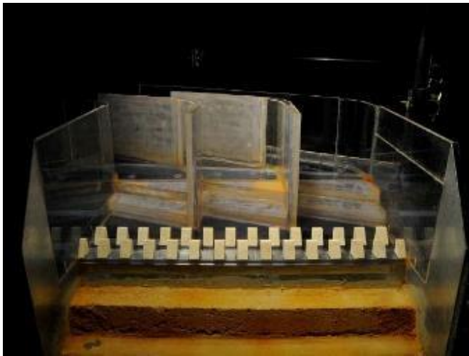
5 : Configuration of the baffle blocks
