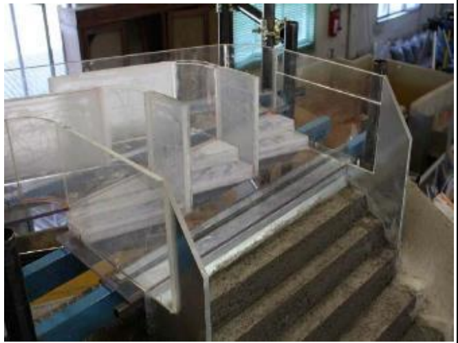
4: Channel bend and the first steps of the stepped chute
