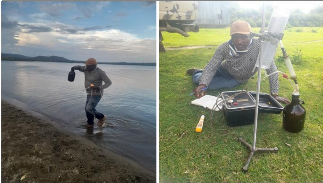
Figure 3.6 Radon measuring on site
