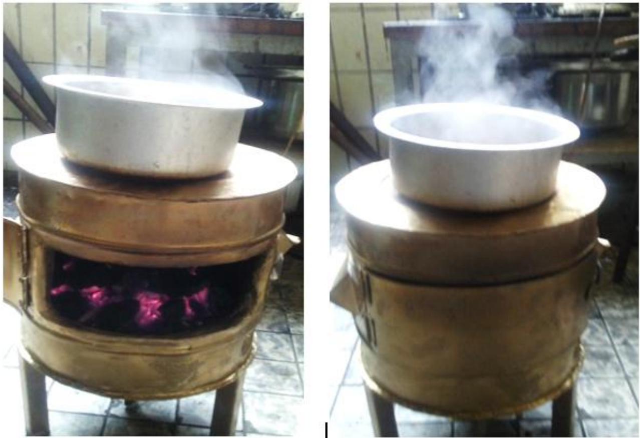
Figure 4.15 Experimental set up for water boiling test
