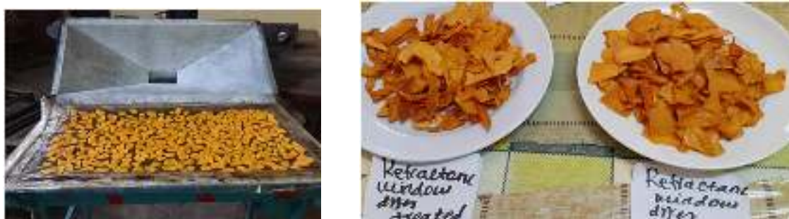
Figure 13; Papaya drying with refractance window and its dried product
