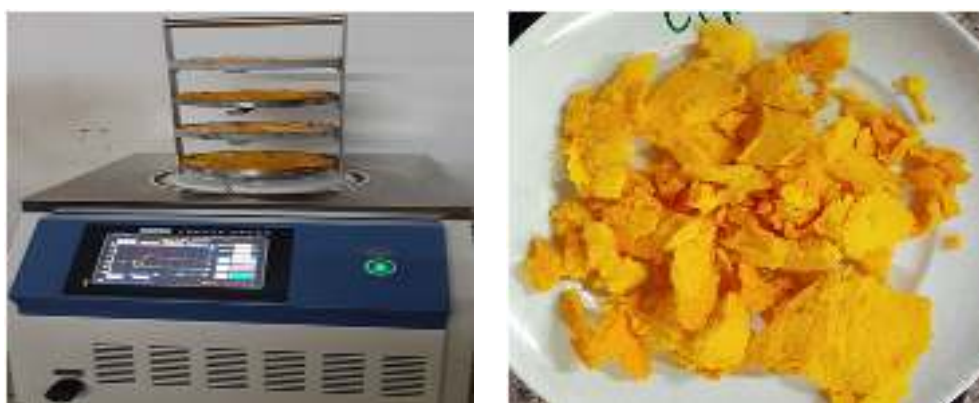
Figure 14; Papaya drying with freeze drier and its dried product
