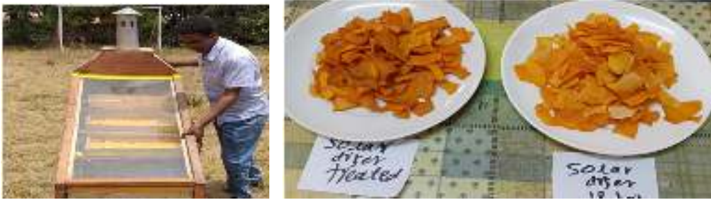
Figure 10; Papaya drying with solar-tray drier and its dried product
