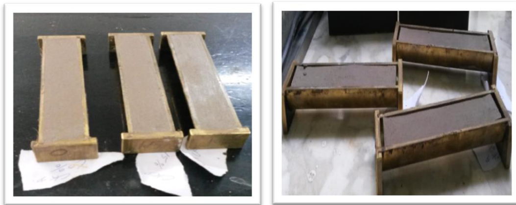
Figure 4.11 Specimen on Air drying Process with varying percentage of CKD
