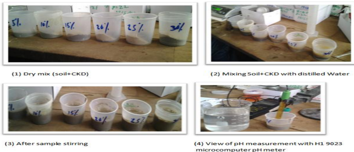
Figure 4.18. View of pH value Determination Lab Procedure
