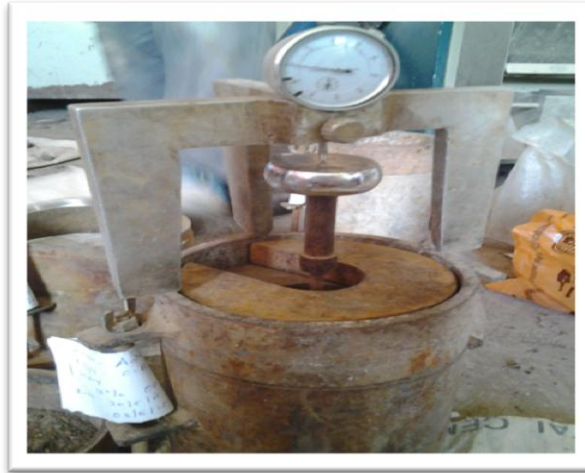
Figure 4.10 CBR Swell Dial Reading Process
