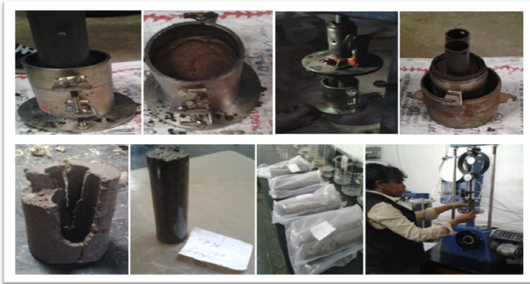
Figure 4.13 Unconfined Compressive Strength Test Process
