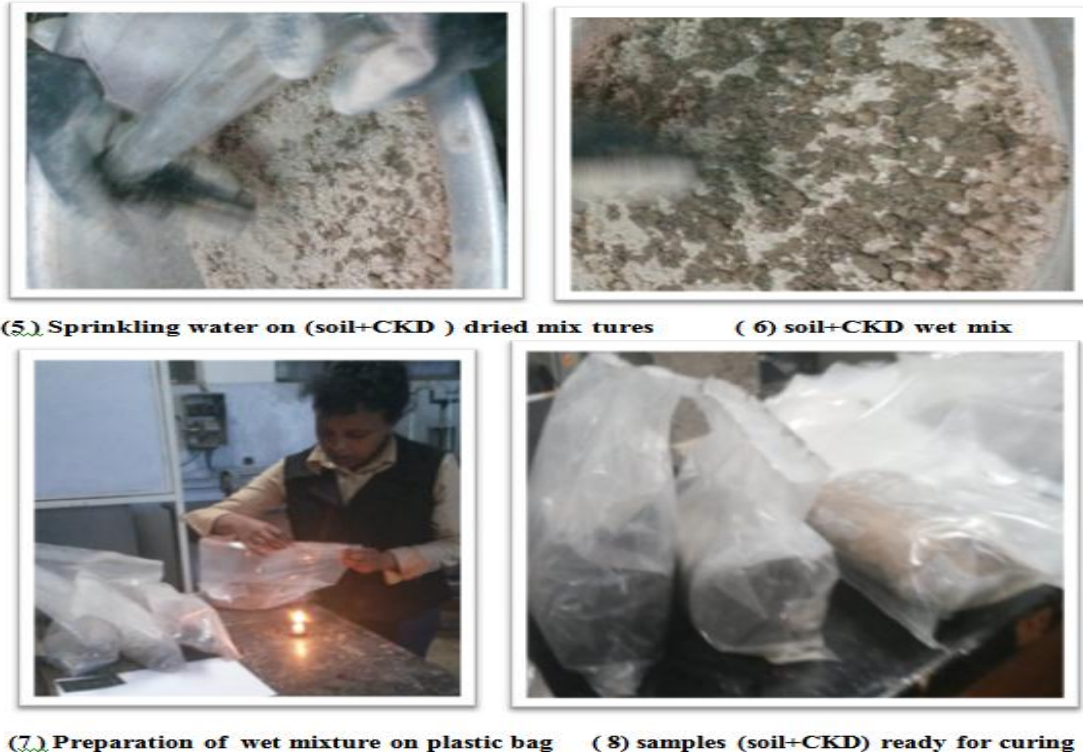
Figure 4.20 Soil-CKD Mixing Procedure
