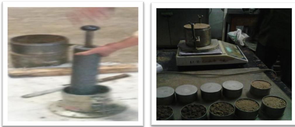
Figure 4.6 Standard Proctor Test on progress
