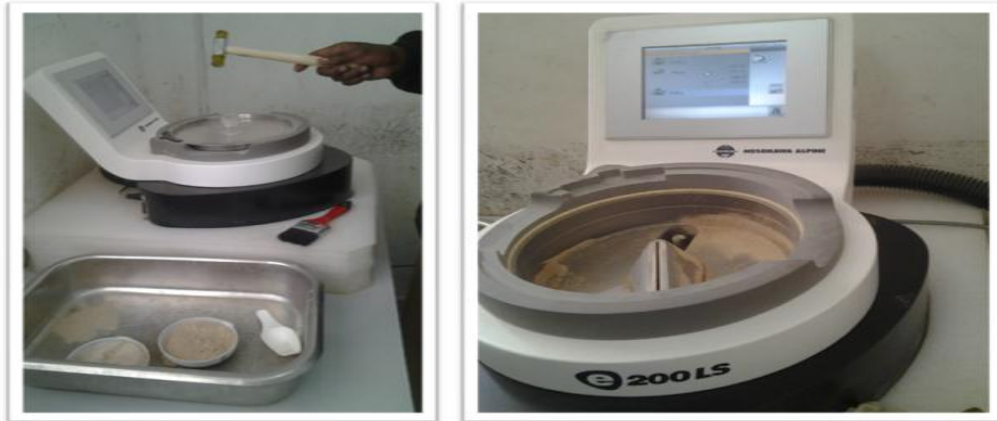
Figure 4.17 View of CKD Physical Analysis Test at MEC Laboratory
