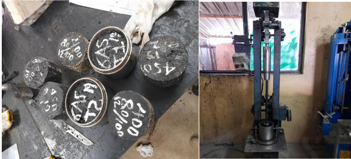
Figure 3.6 Marshal Test Machine and Compacted Specimens
