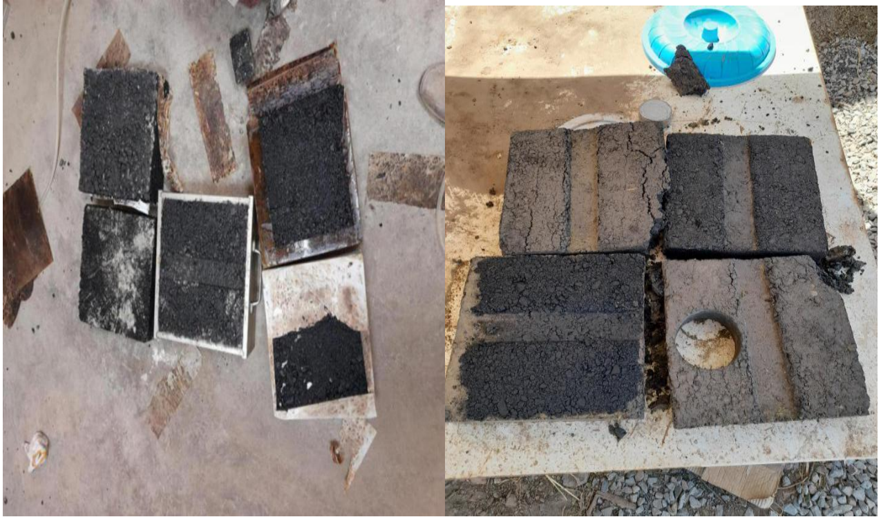
Figure 3.9 Asphalt specimens after wheel tracking test
