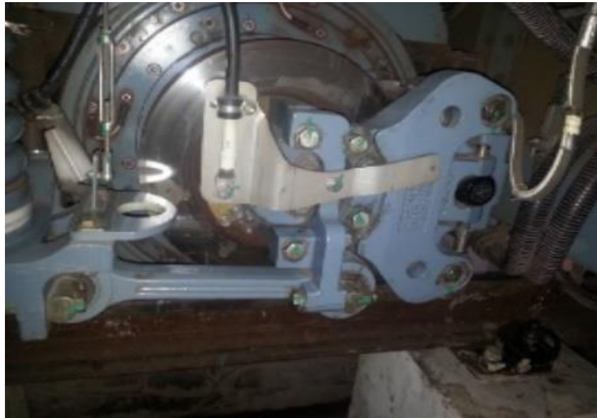
FIGURE 15: THE BRAKING SYSTEM OF THE ROLLING STOCK
