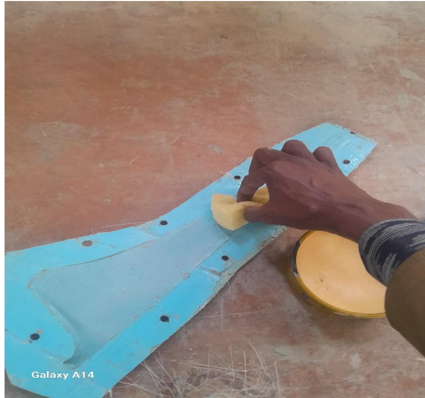
Figure 5.6: - Mold surface preparation applying JELCOAT and PVA for Release Purpose
