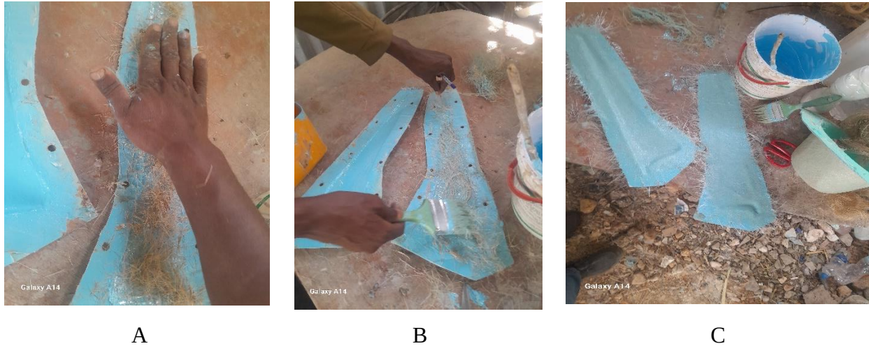
Figure 5.7: - A=Fiber preparation, B= Resin application on Fiber, C= Completed Layer of Blade half
