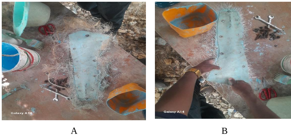
Figure 5.8: - A= Mold half's joining, B= Mold Half connecting by bolts
