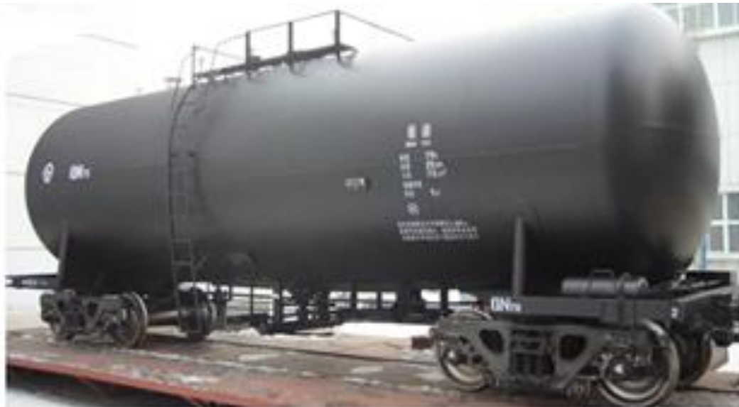
Fig. 3-2.a. Real appearance of GN-70 fluid freight wagon [ERC]
