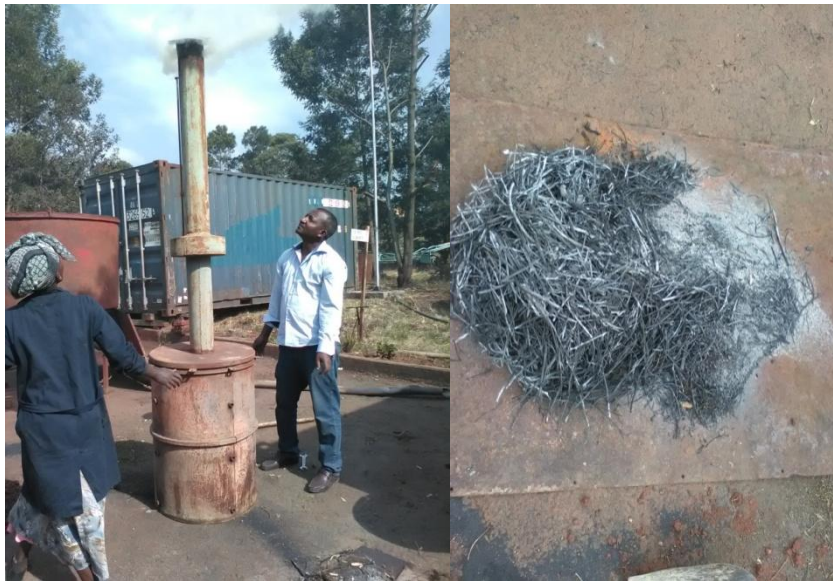
Figure 4c: carbonization of khat waste in barrel kiln and it result
