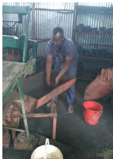
Figure 6c: Binding of charcoal with binder and manufacture of briquette (beehive machine)
