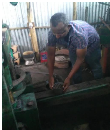
Figure 6c: Binding of charcoal with binder and manufacture of briquette (beehive machine)
