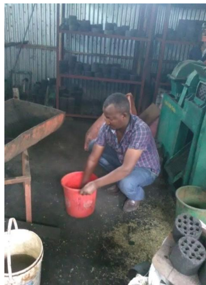
Figure 5c: Grinding and binder preparation for briquetting
