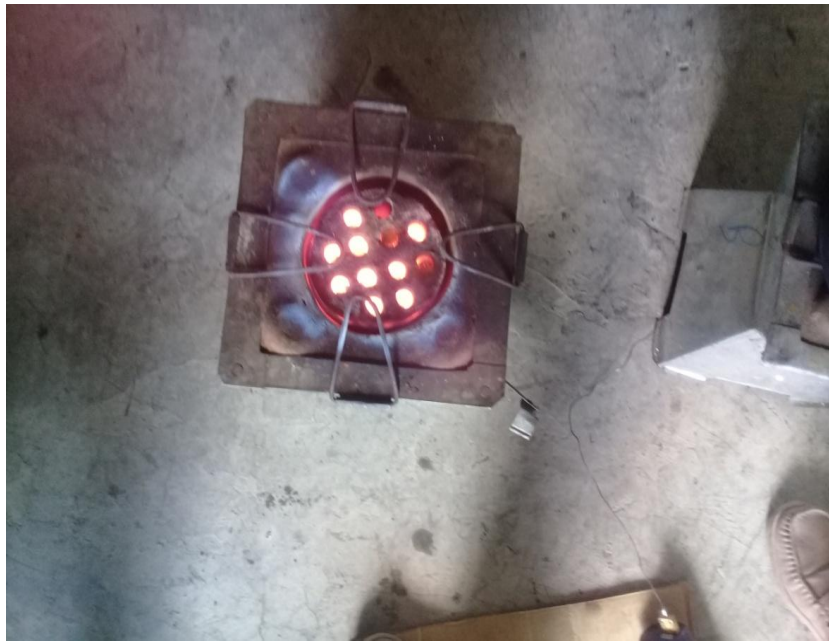
Figure 3d: sample preparation and boiling test of khat waste briquette
