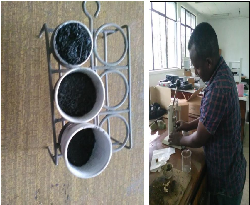
Figure 1d: sample preparation for moisture content, volatile mater, ash content and calorific value measurement.
