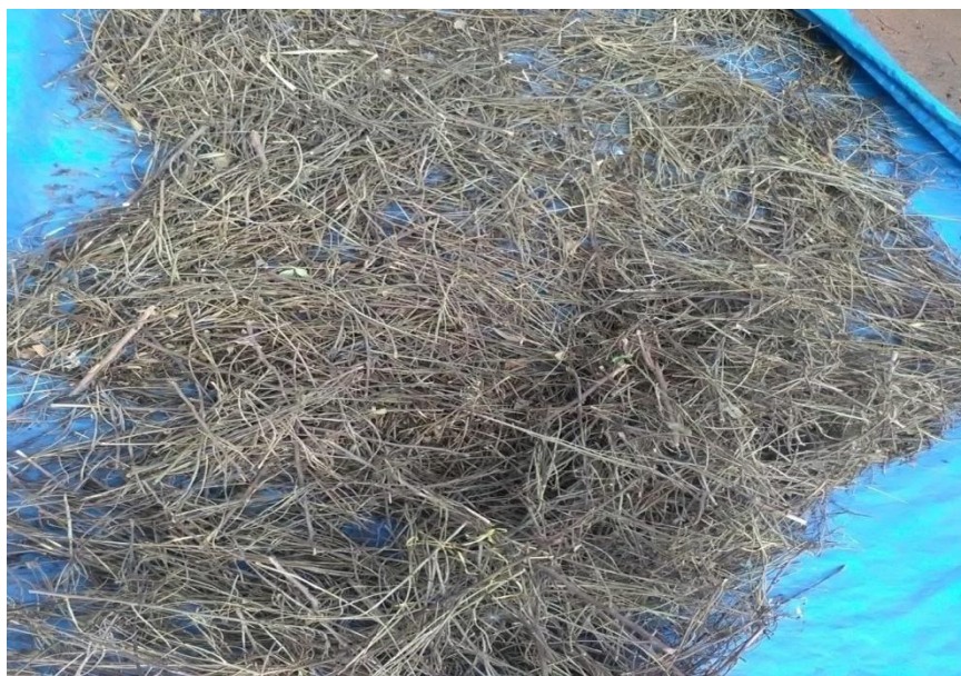
Figure 1c: air-drying of sample for briquette production
