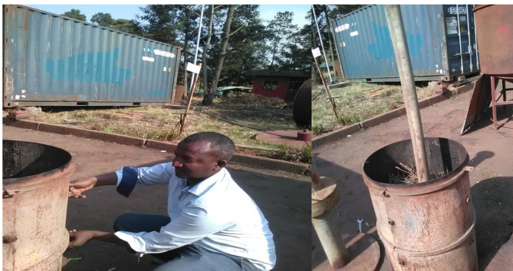
Figure 2c: kiln preparation and wastage addition to kiln for combustion.
