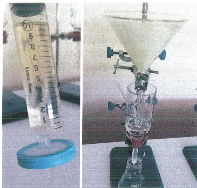
Figure 2: A/ Glass syringe barrel in which its tip was fitted with 0.2 \mu\text{m} filter disk; B/ Immune affinity column fitted with filter paper.
