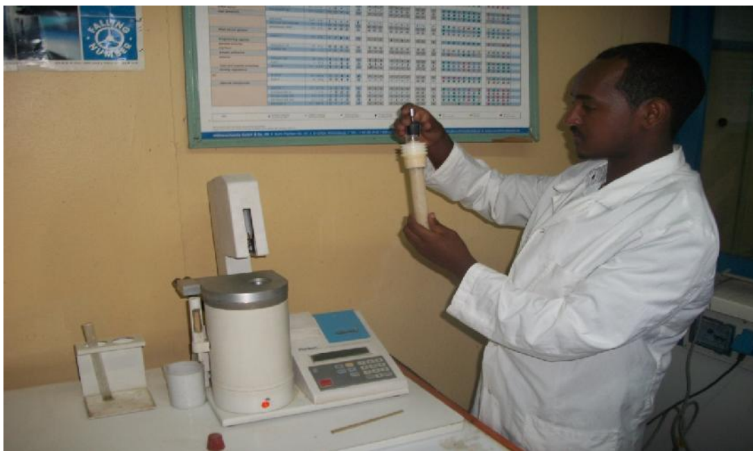
Figure 3.5: Falling Number measuring instrument (Perten Instruments, Sweden , 2005)
