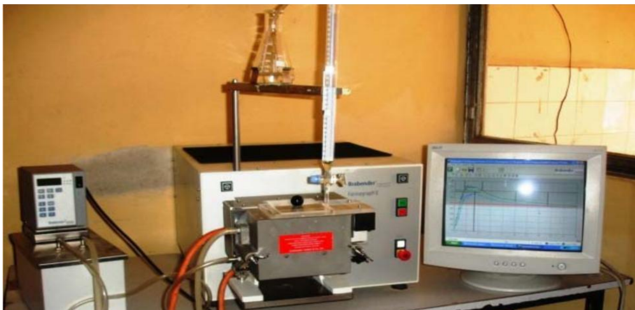
Figure 3.3: Farinograph measuring instrument (Brabender, Germany)
