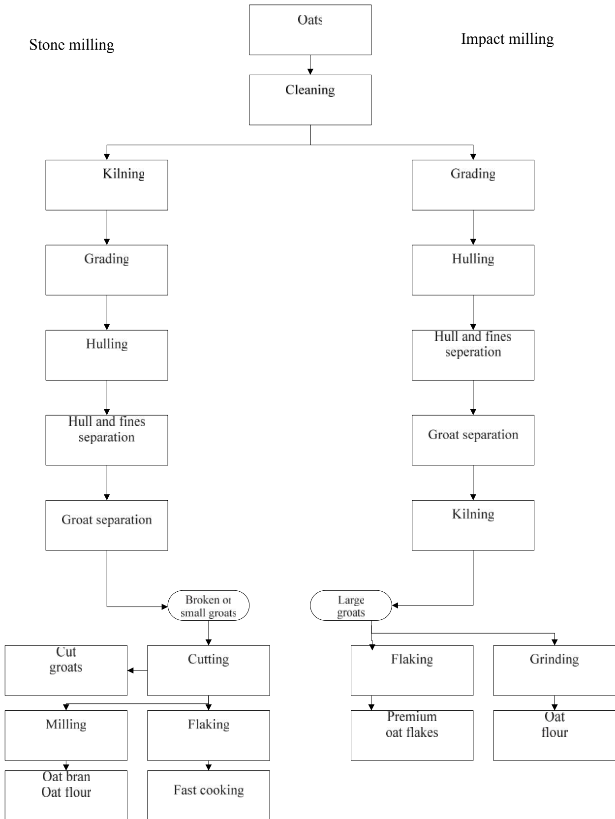
Figure 2.4: The milling process of an oat kernel
