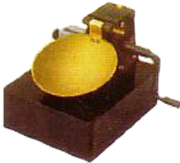
Figure A- 1 Hand operated liquid-limit device
