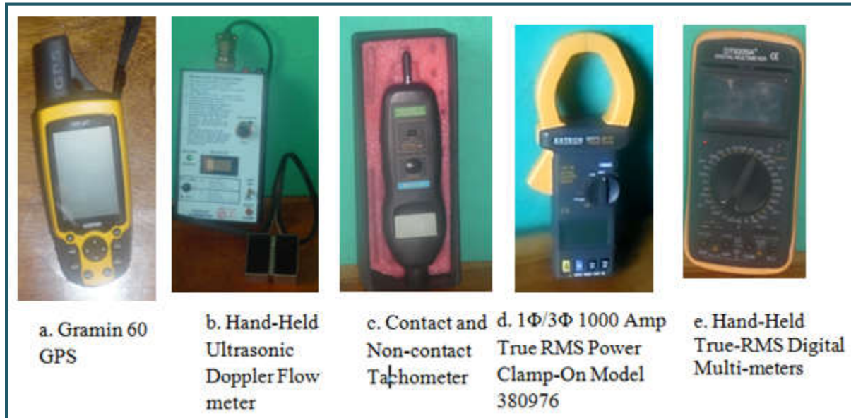
Fig.3. 3: Equipments used during the performance test of Walga MHPP
