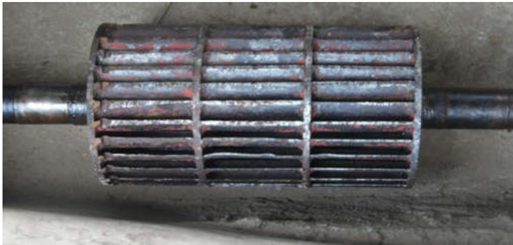
Fig.1.4: Locally Manufactured Cross-flow Turbine
