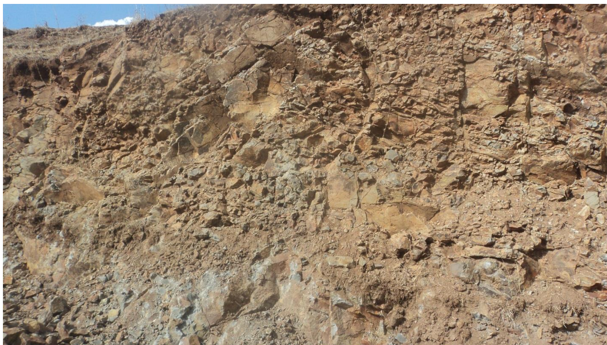
Figure 5-1 Weathered and fractured Tarmaber Amba Aiba basalt from the Middle of Berga river catchment
