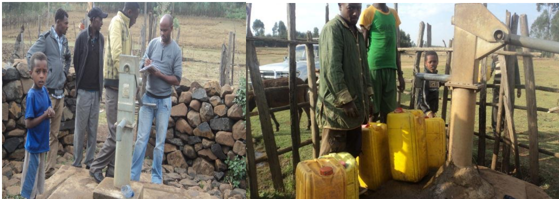
Figure 7-5 hand pump type Indian mark II Afridev pump
