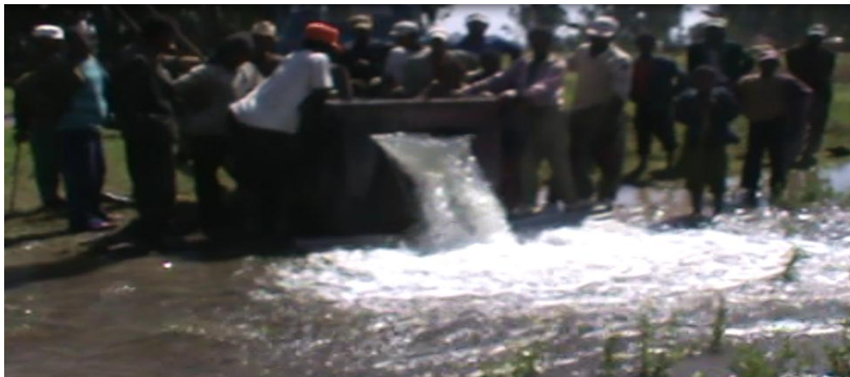
Figure 5-4 BTW-01, during pump test with Q=62.5 l/sec.
